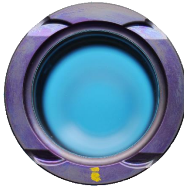
Figure 6-17 Design of glass piston for transparent engine
