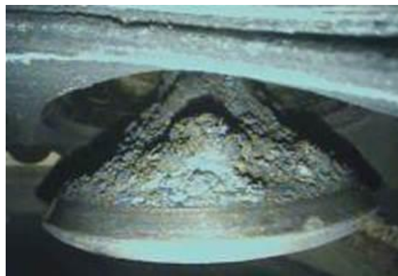
Figure 5-11 Deposits on intake valve
