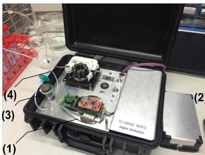
**Figure S4-1:** Final laboratory setup for the ALPACA. During measurement, the algae module (1) is enclosed in a metal housing (2) to prevent interferences from ambient light or electromagnetic field (EMF) radiation. The valve on the inlet (3) changes between an optional filter inlet for rinsing and the sample inlet. The pump (4) is placed behind the outlet to ensure continuous flow.
