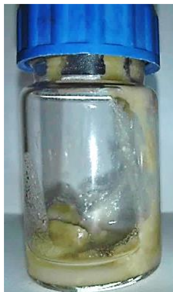
Figure 63 Acid catalyzed OEE product mixture starting with DMM and TRI as educts after neutralization with ethanolic NaOH
