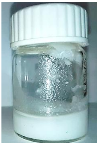
Figure 62 Acid catalyzed OME product mixture starting with DMM and TRI as educts after neutralization with aqueous NaOH
