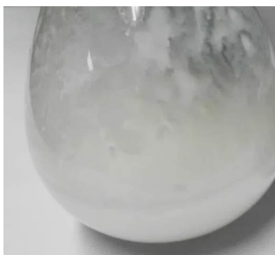
Figure 56 Reaction performed under N 2 pressure; reaction conditions: n DMM /n TRI = 1, 1.0 wt% H 2 SO 4 , t = 60 min; 80°C, 9.0 bar N 2
