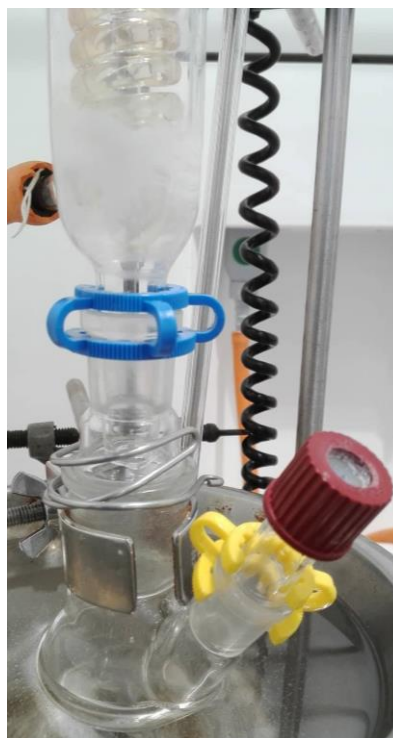
Figure 30 Reaction set-up; glass cuts secured with plastic or metal clips; openings are sealed with rubber septum or glass stub; external temperature control of the paraffinic oil bath; tubes for water cooling of the reflux condenser;
