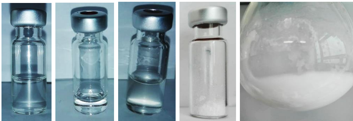
Figure 71 (from left to right) (a) DMM (98% purity), (b) OME 2 (97% purity), (c) OME 3 (96% purity with small amount of OME 4 ), (d) pFA and (e) OME 8-12
