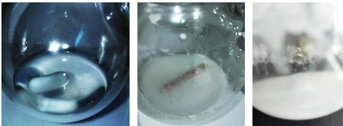
Figure 44 From left to right: OME reactions catalyzed by 2.0 wt%, 3.0 wt% and 3.8 wt% MSA loading (reaction conditions: 80°C, 60 min, n DMM /n TRI = 1)
