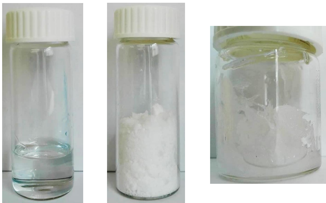
Figure 72 Left: OME 2-7 products upon single-step distillation; middle: colorless solid residual upon single-step distillation containing OME 8-12 , neutralization precipitate and pFA; right: TRI in small amount of OME product
