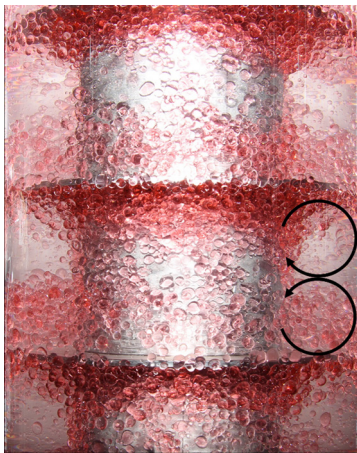
Figure 1. Dispersed-phase distribution at 450 rpm and phase ratio 1. Shaft diameter: 0.05 m, rotor diameter: 0.086 m, compartment height: 0.05 mm, column diameter 0.1 m.
