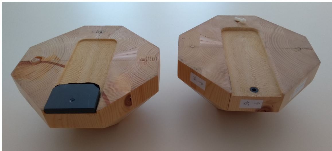
Figure 5.6: Wooden structure, open with visible smartphone insertion
