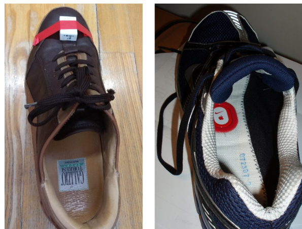
Figure 8.1: Left: Foot-mounted module used, Right: Nike+ shoe and transmitter
