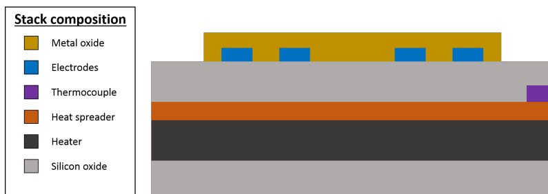
Figure 3.7.: Schematic representation of a cross-section of the membrane stack with its general layer composition.
