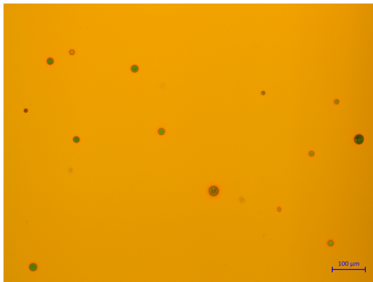
Figure 4.20.: Light microscopy picture of zinc oxide thin film deposited by spray pyrolysis at 400°C. Precursor solution: zinc acetate in mixture of water and ethanol (1:3)
