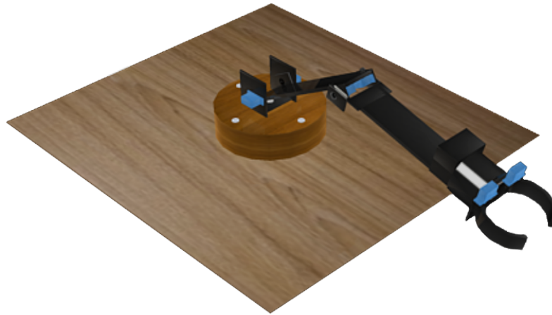
Figure 5.5.: Initial 3D design for the robot arm using AutoCAD.
