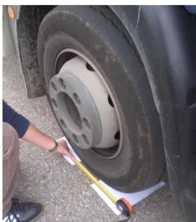
Figure 133: simple measuring method for getting the accurate wheel contact patch geometry
