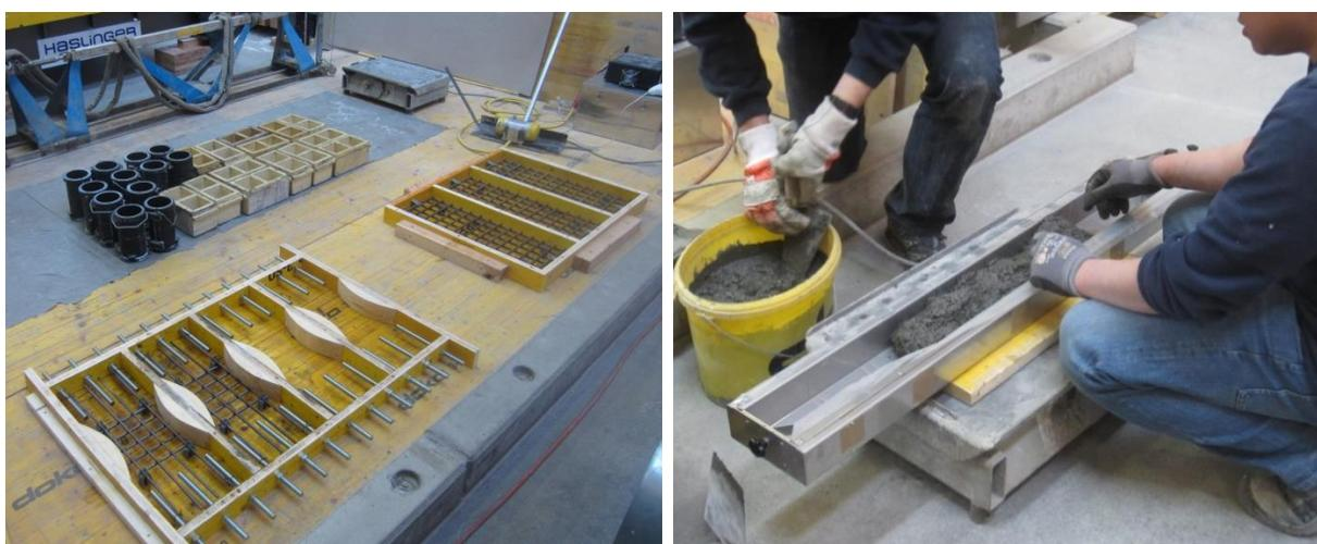
Figure 253: test specimens for accompanying material tests referring to the UHPFRC
