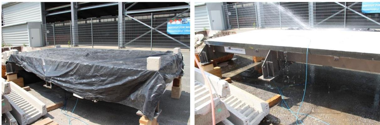
Figure 258: storage of the test specimen outdoors and – left: covering the test specimen with a black foil; right: sprinkling the concrete surface with water
