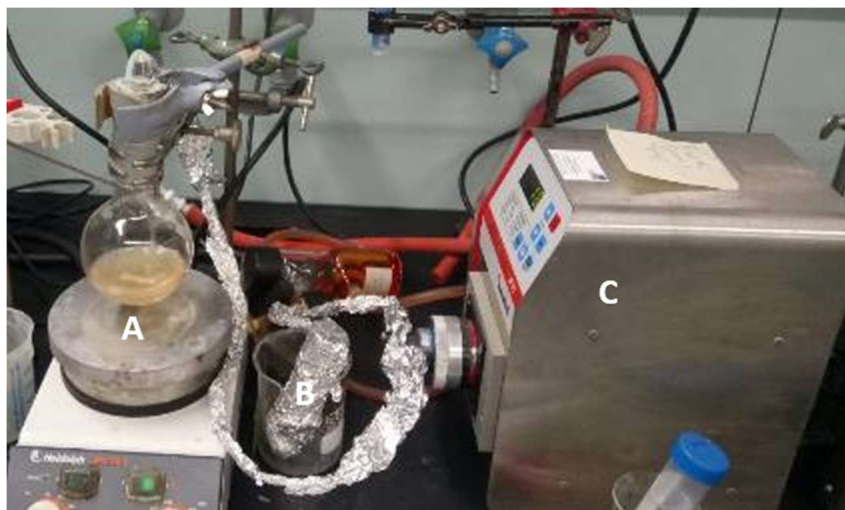
Figure 10 Reaction set-up for prep-scale conversion of fatty acids with P450 J \alpha utilizing a pump for automated \text{H}_2\text{O}_2 pulsing. A = reaction vessel with P450 J \alpha and substrate. B = \text{H}_2\text{O}_2 stock solution (200 mM). C = Pump system.
