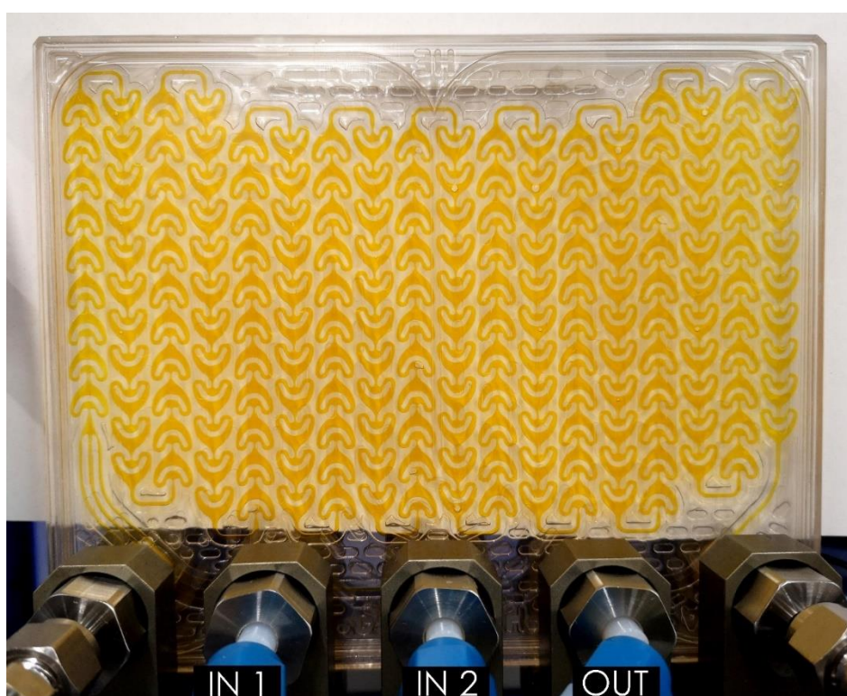
Figure 4. Photograph of the reaction plate with heart-shaped mixing elements. Reaction channels highlighted in orange using aq. bromine solution.
