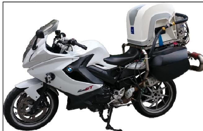
**Figure 5.1:** Experimental setup of the PEMS device on the test vehicle [4.11].
