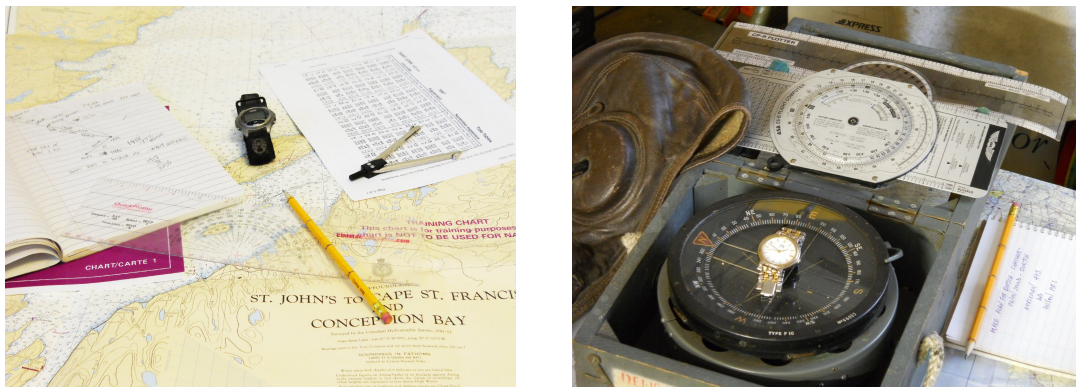
Figure 2.2: Left: Dead reckoning navigation tools in coastal navigation. Right: British P10 Magnetic Compass with dead reckoning navigation tools. (Bond, 2013)
