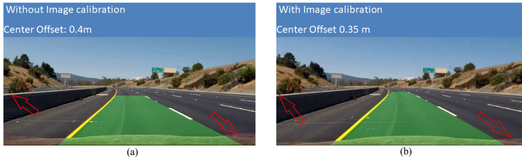
Figure 4.7: Distortion effects on image perception, calibration done via OpenCV API.
