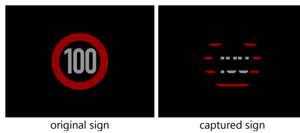
Figure 5.37: LED flicker effect, frequency = 250\text{ Hz} duty\ cycle = 20\% .
