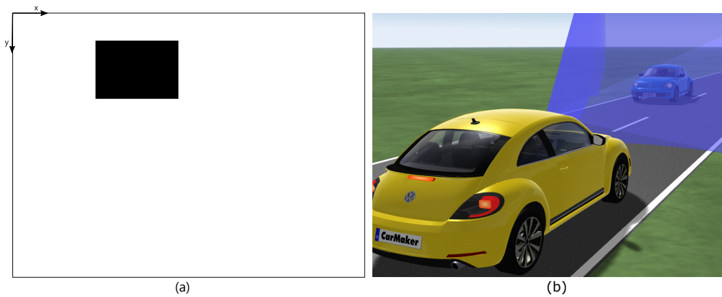
Figure 5.33: (a) bounding box representation of detected vehicle without the rolling shutter effect, (b) corresponding virtual scenario.
