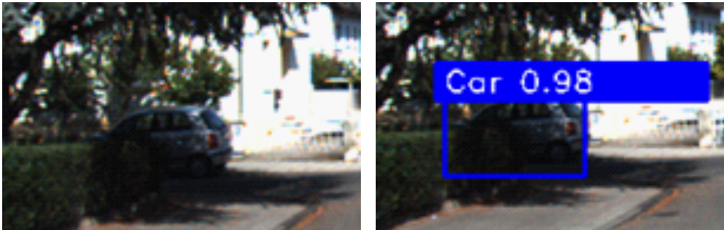
Figure 7.22: Detected car under low illumination by the DNN trained on the augmented dataset (right figure).
