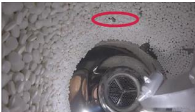
Figure 73: Maritime BioLogger inside the tablet bed in the ConSigma® 320 tablet coater.
