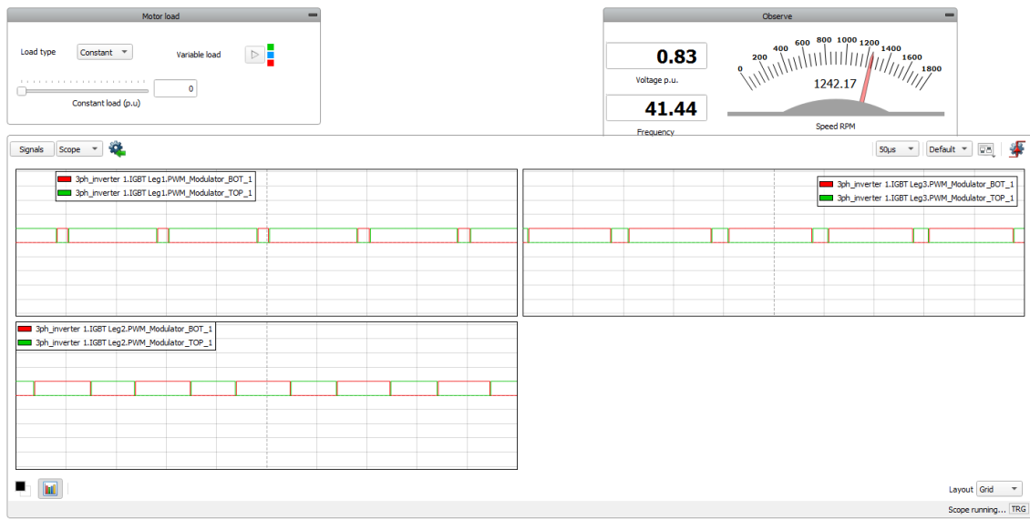
Figure 6.8: Inverter legs PWM control signals
