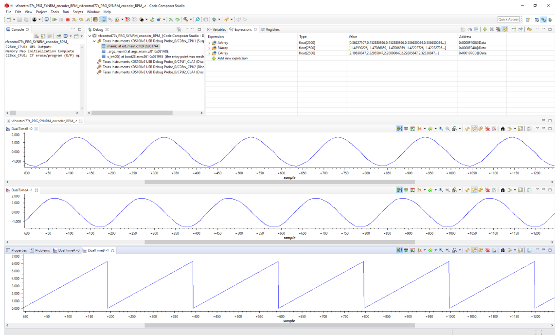
Figure 8.6: Stator currents and rotor angle measurement with Code Composer Studio
