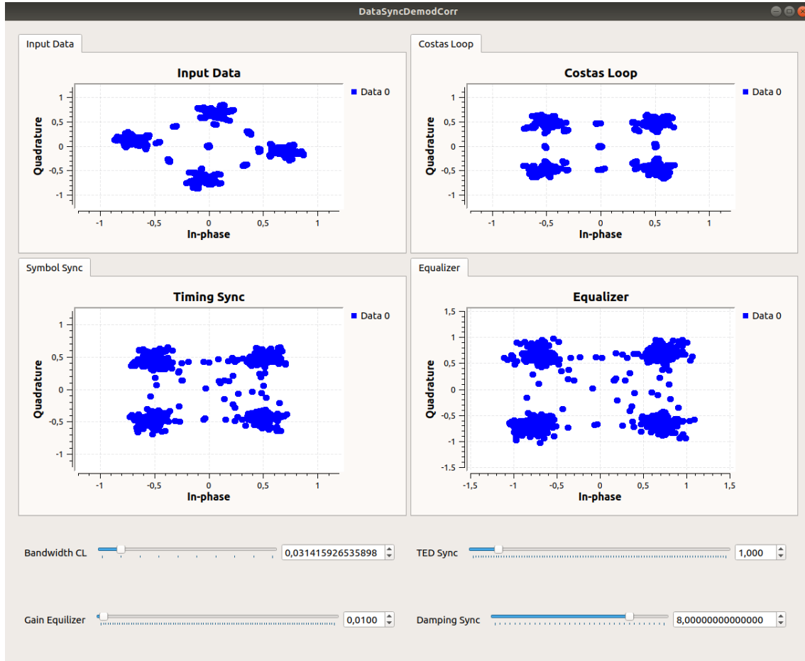
Figure 8.12: Results of the received samples when using only one LimeSDR as TX and RX simultaneously.
