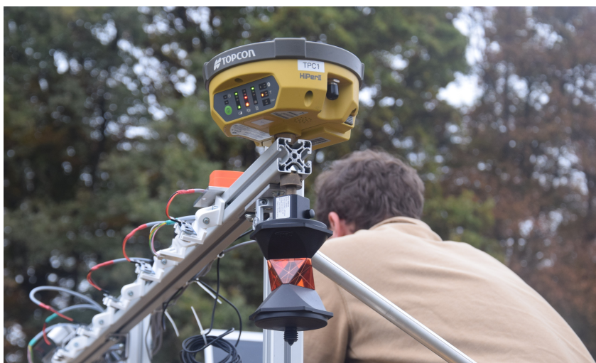
Figure 7.1: Leica 360°Mini Prism mounted below geodetic GNSS receiver
