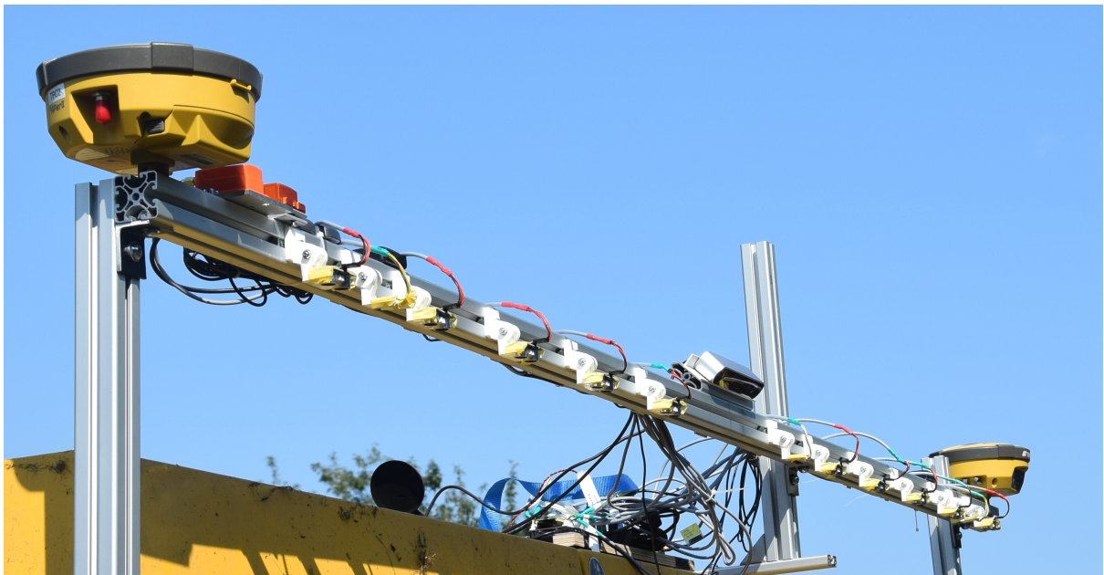
Figure 5.1: Aluminium profile with mounted sensors; GNSS receivers (yellow) + IMU (orange) mounted on the sides for reference data generation; stereo camera and other DME mounted inbetween
