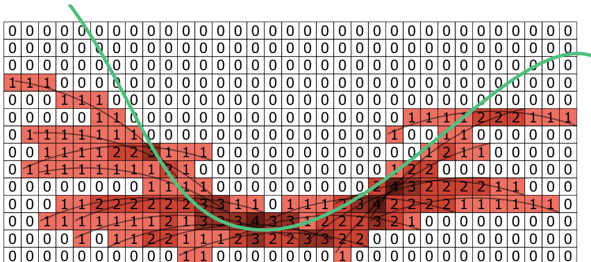
Figure 2.3: Spatial voting scheme pixel representation of example scene with measurement uncertainty arcs (black) and the true surface representation (green); Pixels contain the sum of the number of arcs which coincide with them; pixelated surface profile approaches real profile with increasing number of measurements
