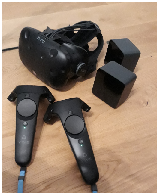
Figure 5.2.: HTC Vive HMD with controllers and base stations.
