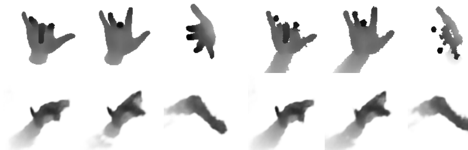
Figure 5.11: Example view predictions for real and synthetic input. Top: Three corresponding synthetic (left) and real (right) validation images. Bottom: Predicted views for synthetic (left) and real (right) input.
