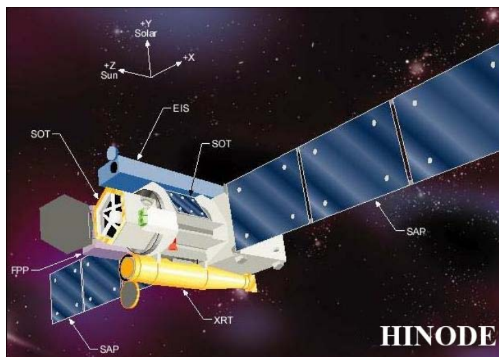
Figure 5. Hinode sensor complement and coordinate system (© eoPortal 2019)
