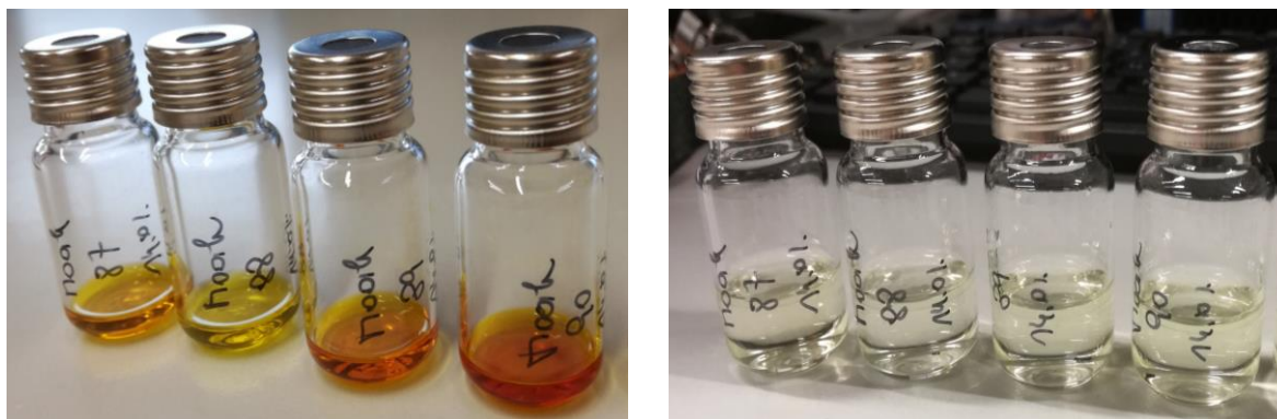
Figure 66: Coloured samples before epoxidation (left) vs. colourless samples after quantitative epoxidation (right).
