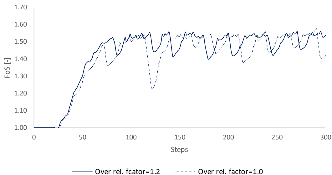
Fig. 51 Influence of the numerical control parameter over relaxation factor on the obtained FoS - \psi'=\varphi'
