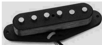
Figure 2.2: The pickup consists of several cylindrical magnetic poles and a coil with a large number of windings wrapped around them. A moving steel string above the magnets causes distortion to the magnetic field, these field-changes are picked up by the coil, which generates the voltage signal.
