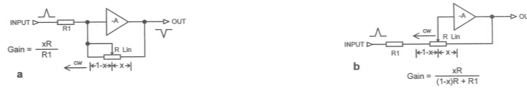
Figure 4.2: This graphic shows two versions of an active gain control and the corresponding gain formula. Each of these two options are very simple and only use one op-amp. The first one (a) has linear gain, while the second one (b) has a somewhat logarithmic gain.
