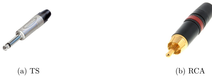
Figure 2.6: The most common connectors for unbalanced input are the 6.3\text{mm} jack plug (a) and the RCA connector (b). The mono jack plug is also called TS. T stands for tip and S for sleeve. The RCA connector is also called cinch connector in other languages.
