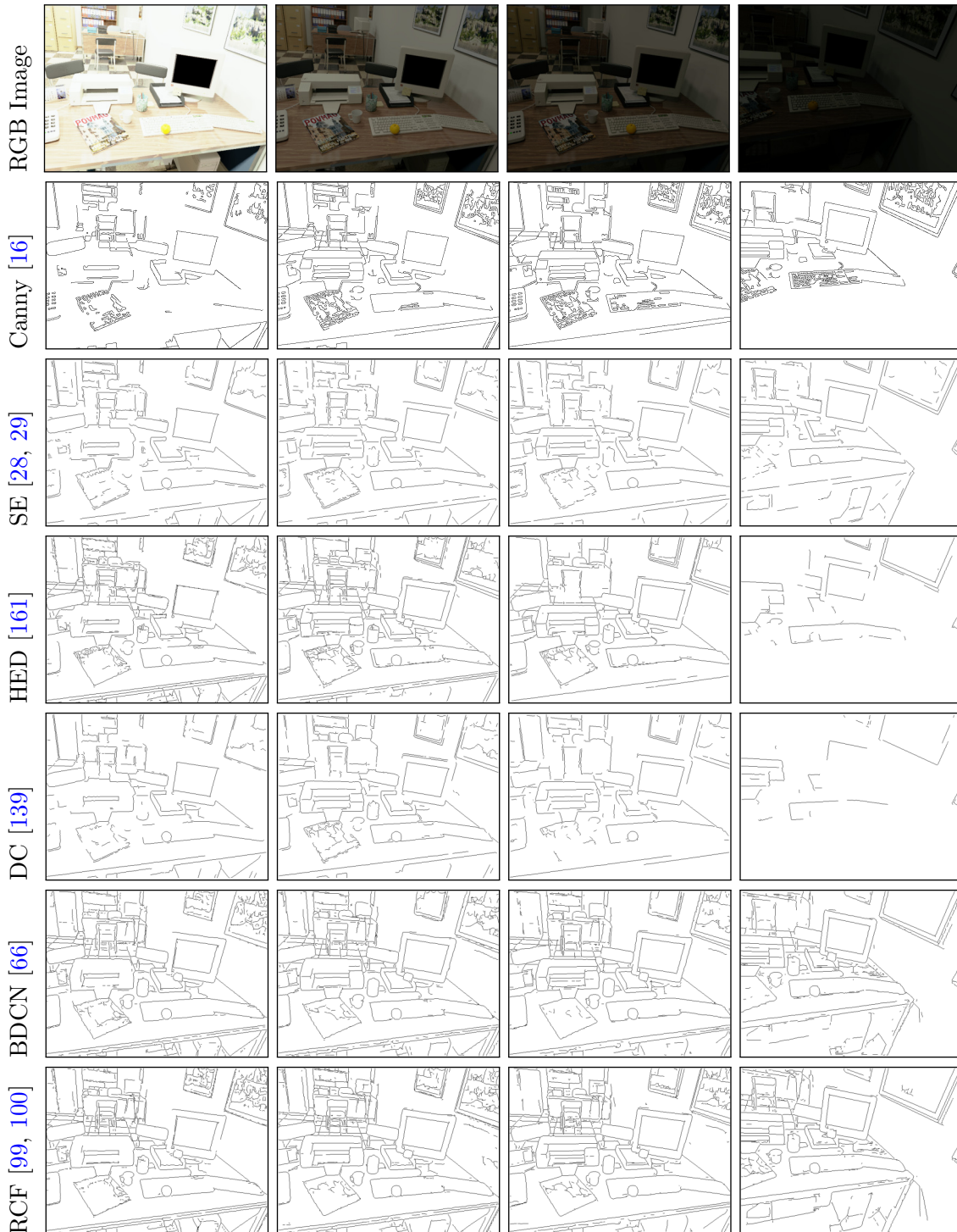
Figure 5.4: Four different RGB images from the HDRFusion dataset [96] with varying illumination and the corresponding edge detections. While all methods work well for the first three images, only SE, RCF, and BDCN deliver relatively constant edge detections even with varying illumination.
