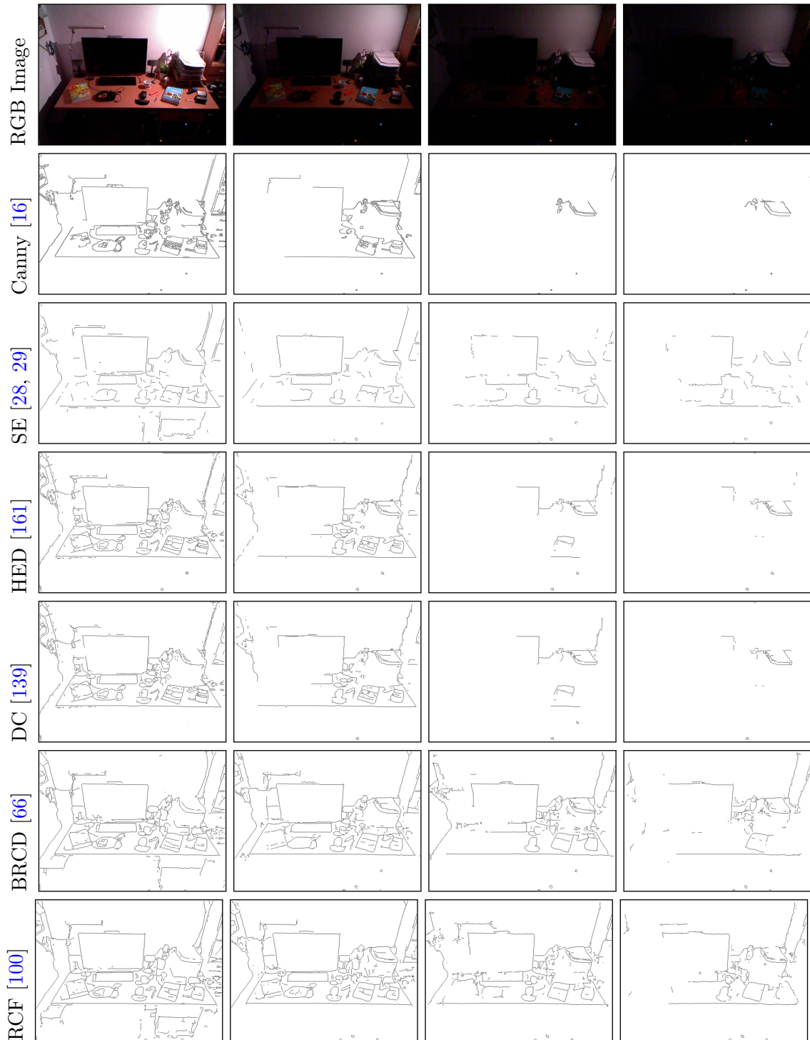
Figure 5.5: Four different RGB images with varying illuminations and the corresponding edge detections. The setup is a static desktop scene with a dimmable light source, which reduces the illumination over several seconds. While all methods work well for the first image images, only SE, RCF, and BDCN deliver relatively constant edge detections even for the second and third image. All detectors fail in the very dark last image.
