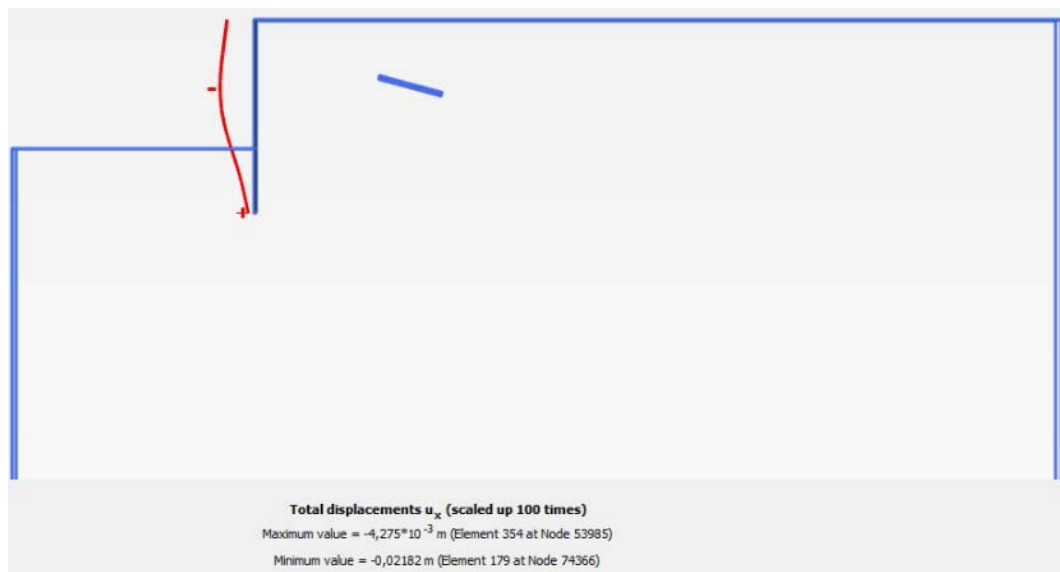
Fig. 172 Deformed sheet pile wall in 3D – volume elements ( E = 2.1E7 kN/m 2 )
