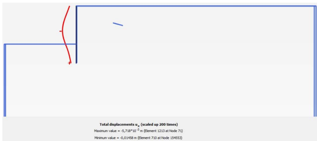
Fig. 261 Deformed sheet pile wall in 2D ( E = 2.1E7 \text{ kN/m}^2 )
