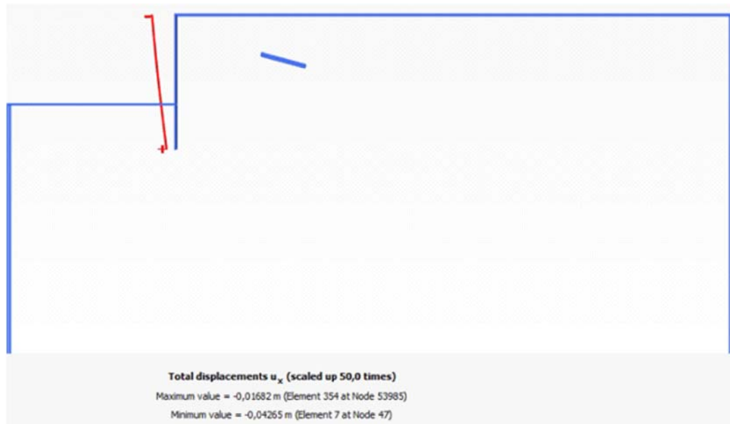
Fig. 290 Deformed sheet pile MC model Soil 2 ( E = 2.1E8 \text{ kN/m}^2 )
