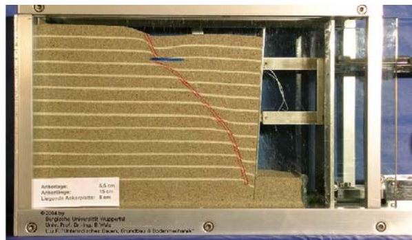
Fig. 37 Lower slip plane with lying anchor plates [23]
