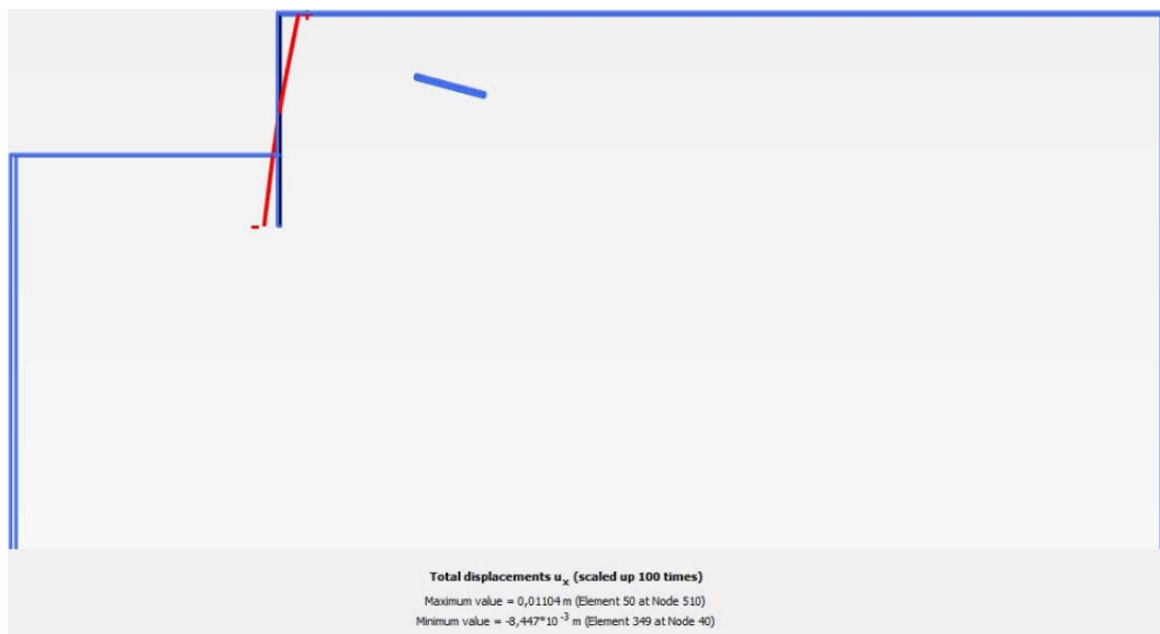
Fig. 275 Deformed sheet pile wall MC model Soil 1 ( P = 100 kN/m)
