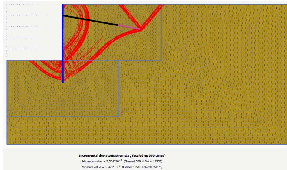
Fig. 111 Incremental deviatoric strain \Delta\gamma_s HS model with Embedded Beam Rows
