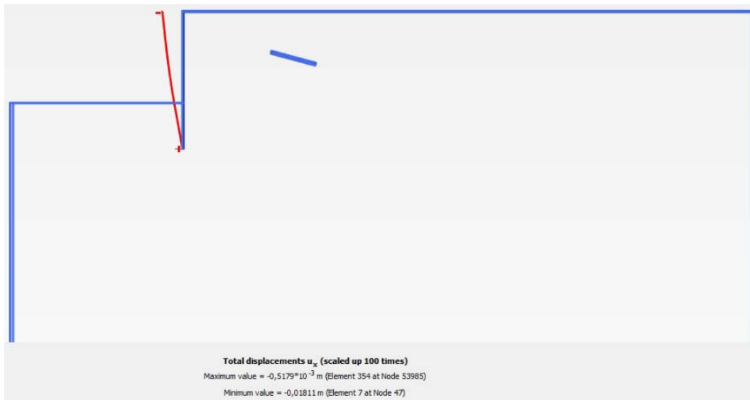
Fig. 303 Deformed sheet pile wall HS model Soil 1 ( P = 100 kN/m)
