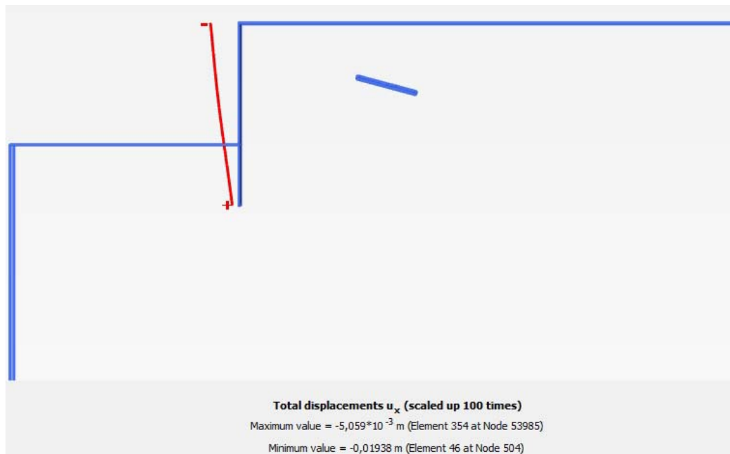
Fig. 203 Deformed sheet pile wall MC model ( P = 0 kN/m)
