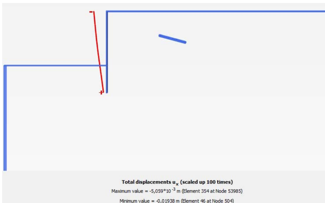
Fig. 289 Deformed sheet pile MC model Soil 1 ( E = 2.1E8 kN/m 2 )
