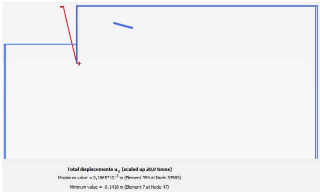
Fig. 246 Deformed sheet pile wall HS model ( E = 2.1E8 kN/m 2 )
