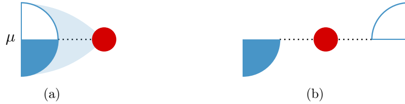
Figure 6.10: (a) Impurity (red sphere) coupled to a partially filled bath (semicircle) at chemical potential \mu . (b) The same hybridization function can be obtained by coupling the impurity to a full and empty bath with appropriate DOS.
