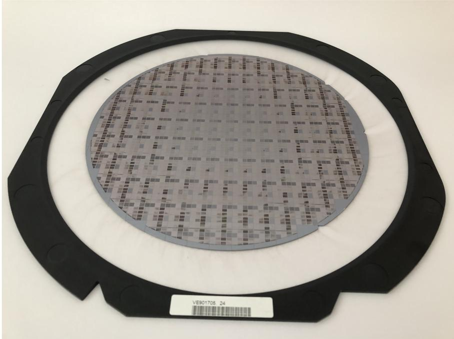
Figure 2.12: Image of a wafer after mechanical dicing. The foil and the frame can easily be seen. The color of the wafer pattern changes, since many pillars are collapsed.
