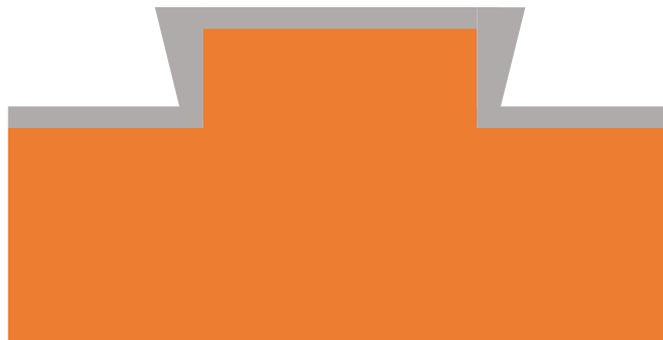
Figure 3.14: For the simulations of the 225 nm and 375 nm deep gratings this overhanging sidewall profile was used instead of straight ones as for the 150 nm deep gratings. Metal/alloy in gray, highly doped poly-silicon in orange.
