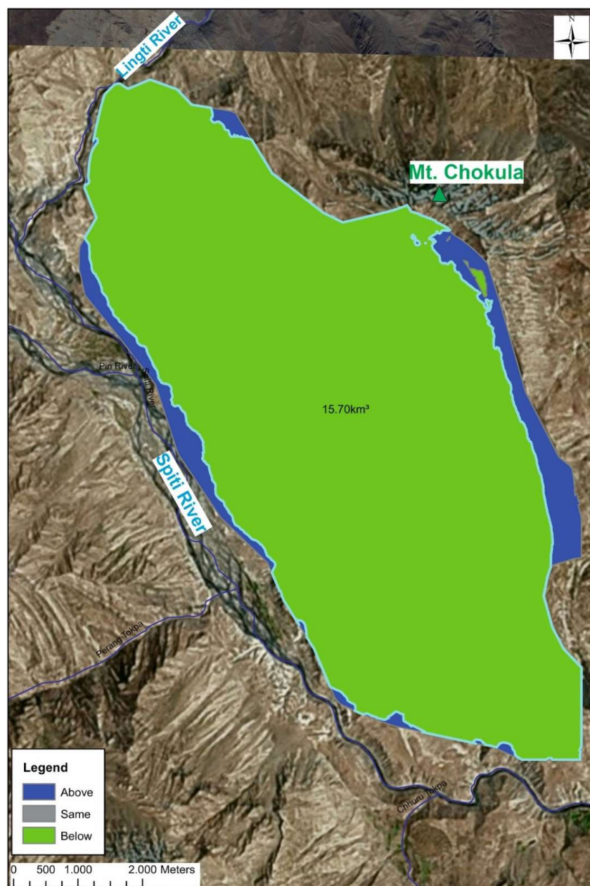
Fig. 4.25 Dangkhar Landslide volume estimate using TIN difference modelling. Modelled volume lies above the basal slip surface (blue) and below the present day surface (green)
