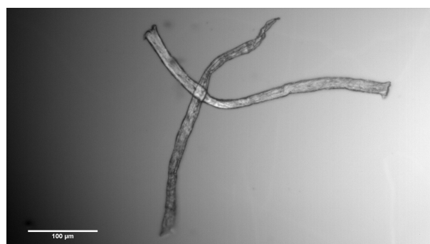
Fig. 21: Optical microscopy image of a typical hardwood FtF-bond with 20x magnification
