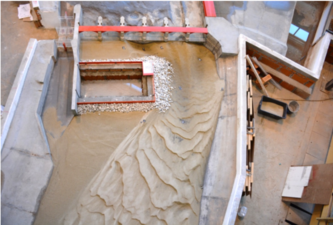
Figure 2.16: Investigation of the sediment transport via physical model study; top: initial state, bottom: final state (Source: Institute of Hydraulic Engineering and Water Resources Management, TU Graz).
