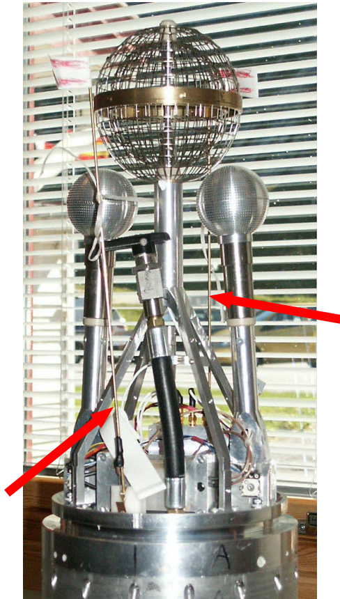
Figure 2.26 Hinged antenna of a MIDAS payload in stowed position (Type 1). The central ion probe uses a gridded collector to allow free airflow (see later, Ch. 3.2).
