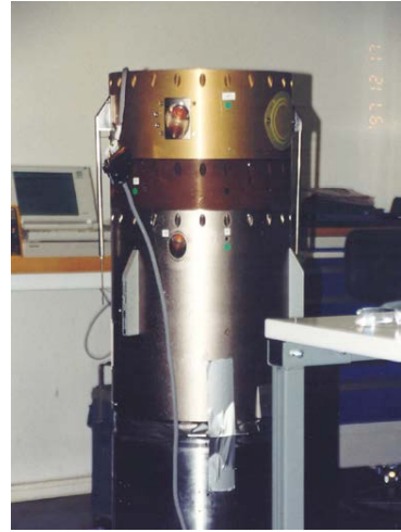
Figure 2.31 Antennas of an NLTE payload for an Orion sounding rocket (Type 6, March 1998, Esrange, Sweden).
