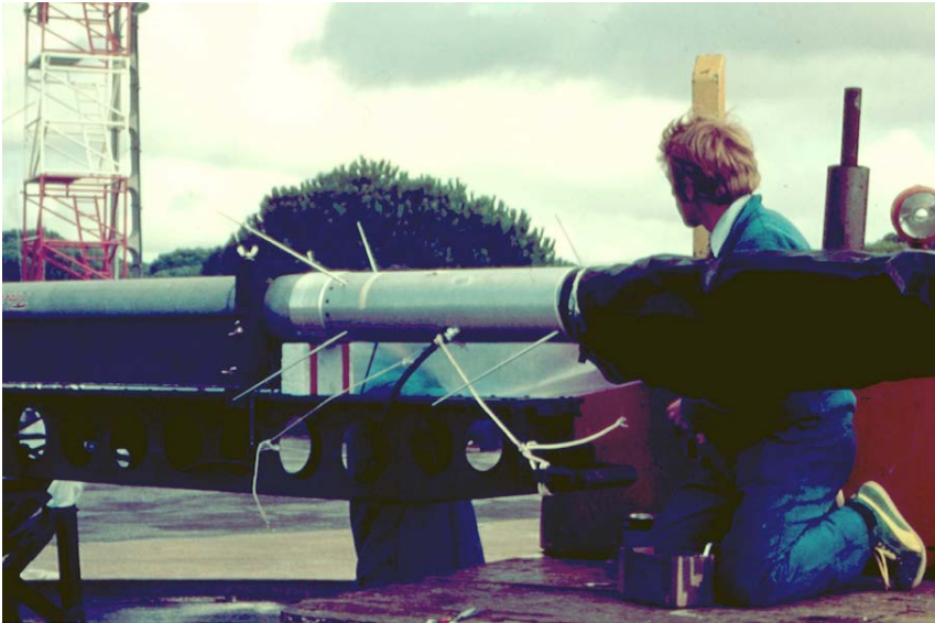
Figure 2.29 Antennas of a payload of an Apache sounding rocket (Type 4, rocket F44, January 1976, El Arenosillo, Spain).
