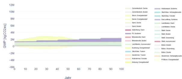
Figure 12: Variant 1 (Low-Tech) LCA study over 100 years life span; dynamic energy mix scenario based on BMU study
