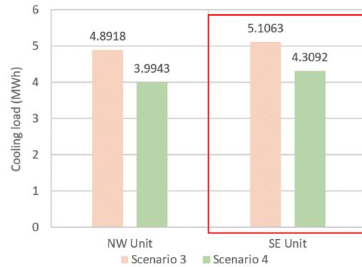
Figure 11: Orientation impact on the annual cooling load
