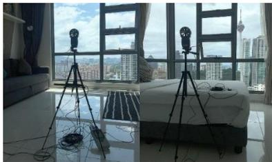
Figure 3: Installation of monitoring equipment in the experimental units
