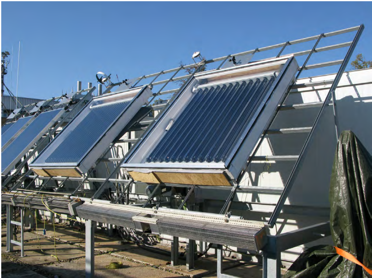
Figure 2: Measures of the façade collector system at the ITW of the University of Stuttgart
