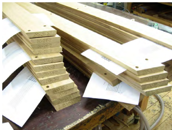
Figure 8: The cladding boards are individually tapered and numbered ( Risør Trebåtbyggeri )
