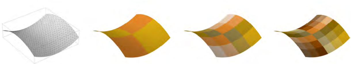
Figure 12: Double in the opposite direction curved Geometry
