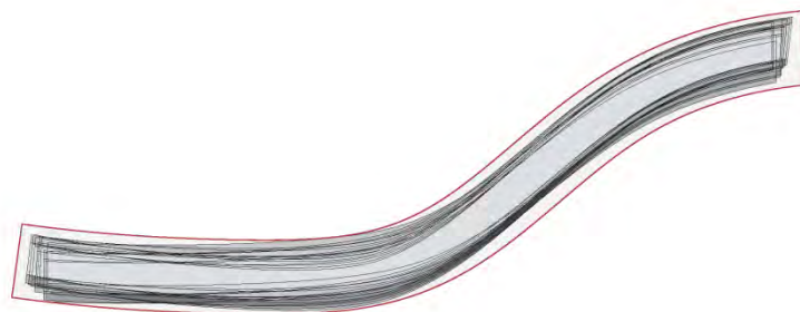
Figure 7: One common timber blank geometry for nine similar, but different beams ( designtoproduction )
