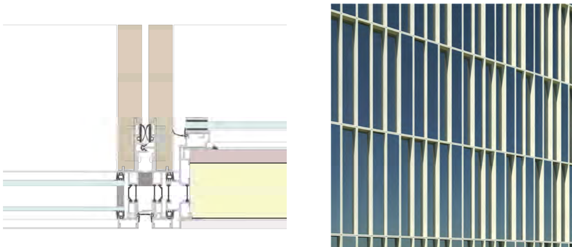
Figure 2: Detailed view of a horizontal cross-section and view in perspective of a possible architectural configuration of the entire FB720 façade system
