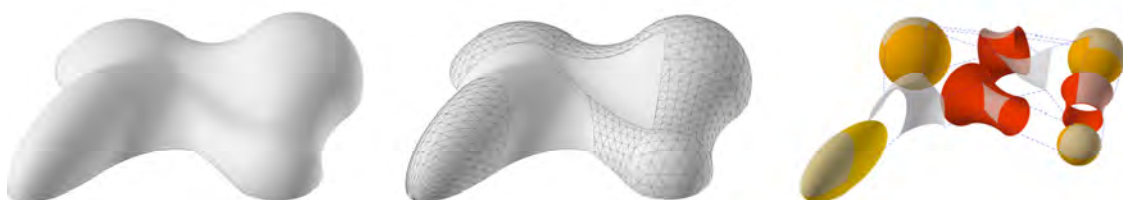
Figure 14: Identification of rule geometries in freeform geometries
