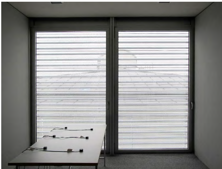
Figure 6: Daylight factor CPC 19%: 1,13%
