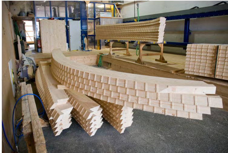
Figure 6: Curved secondary beams with embedded seat cuts for the oak cladding boards ( designtoproduction )
