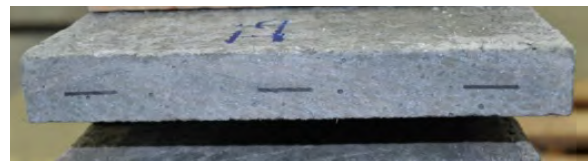
Figure 10: Cross section of the UHPC plate used for test series
