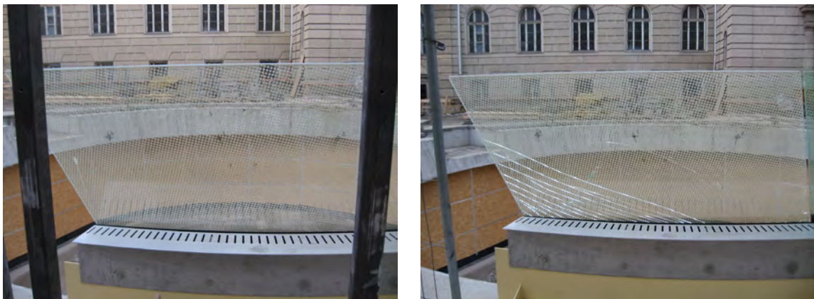
Figure 10: Glass before and after the pendulum impact test [2]
