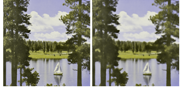
Figure 3. Left: Test image sailboat ( 512 \times 512 pixels) reduced to yellow–blue colour space. Right: Half-space median filtering result, using a discrete disc of radius 2 as sliding window, 5 iterations.
