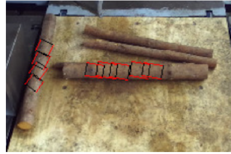
Figure 6. Model logs in the picking area of the 1:5 scaled model crane with marked grasping positions by our AI based method. Red marks the desired locations of the two grippers in the end-effector of the crane.
