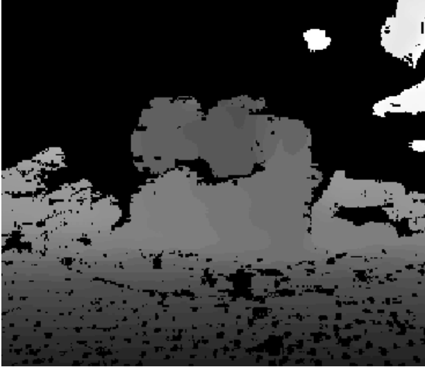
Figure 7. Disparity image of the object viewed by the Intel RealSense camera. Occlusions induced by the stereo vision system make it difficult to accurately locate the grasping area depicted in Figure 1.
