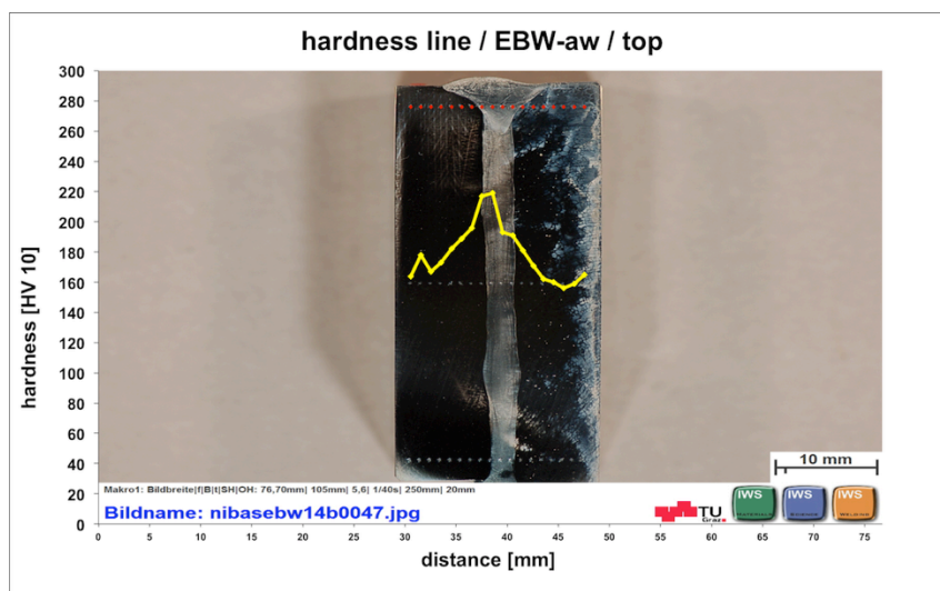
FIGURE 102: HARDNESS LINE EBW-AW TOP
