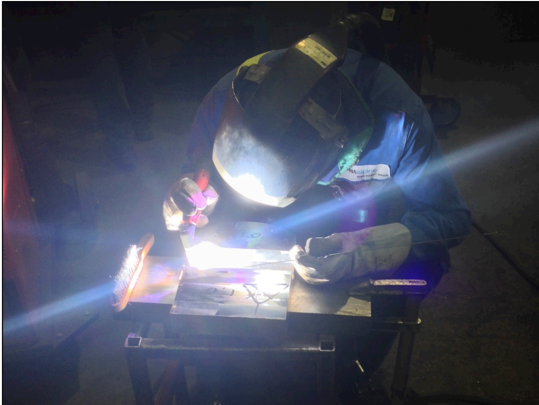
FIGURE 26: TEST-PIECE TIG WELDING AT VAGT
