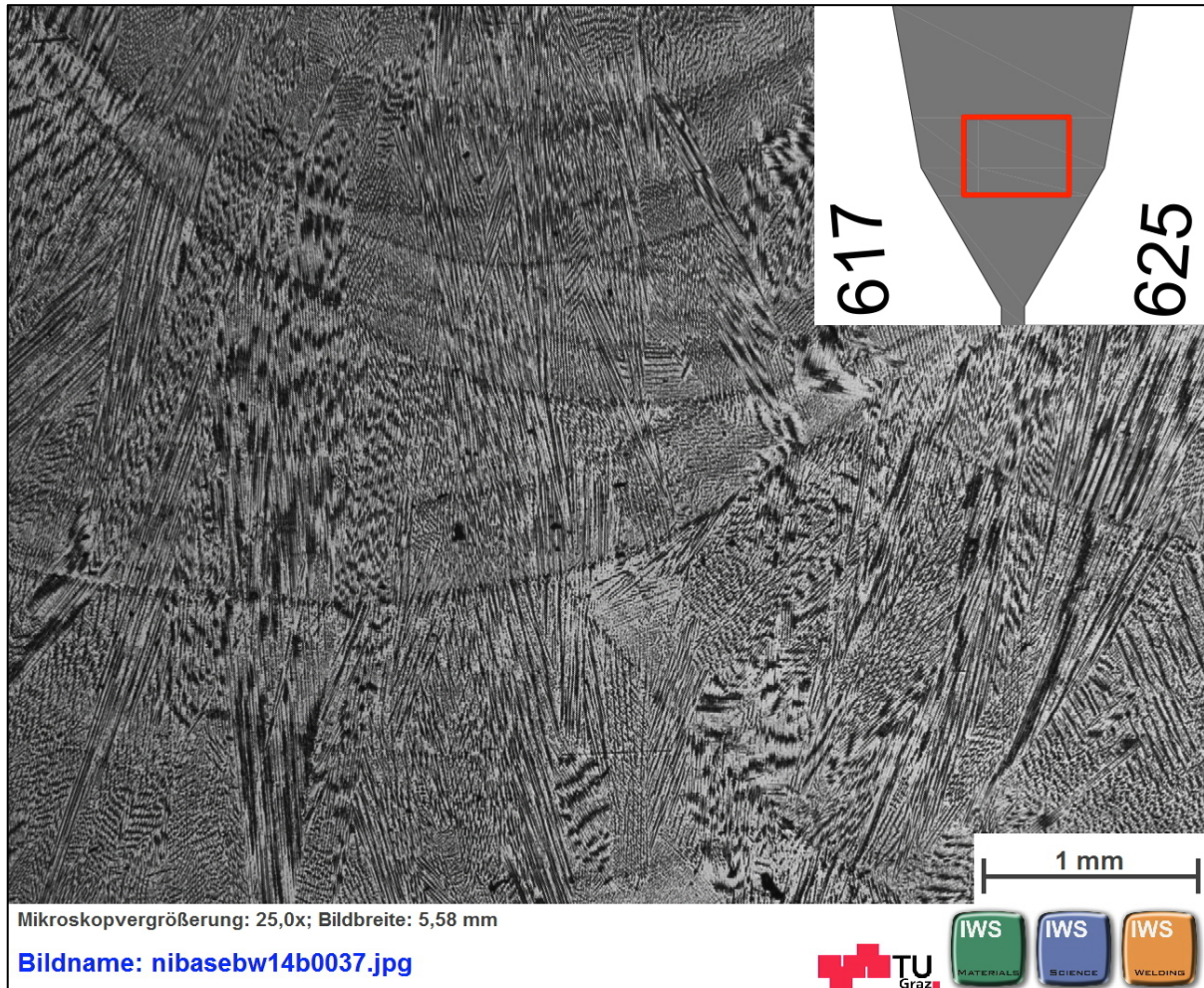
FIGURE 56: LOM IMAGE SMAW-AW WELD METAL ALLOY 625 (V2A ETCHANT)
