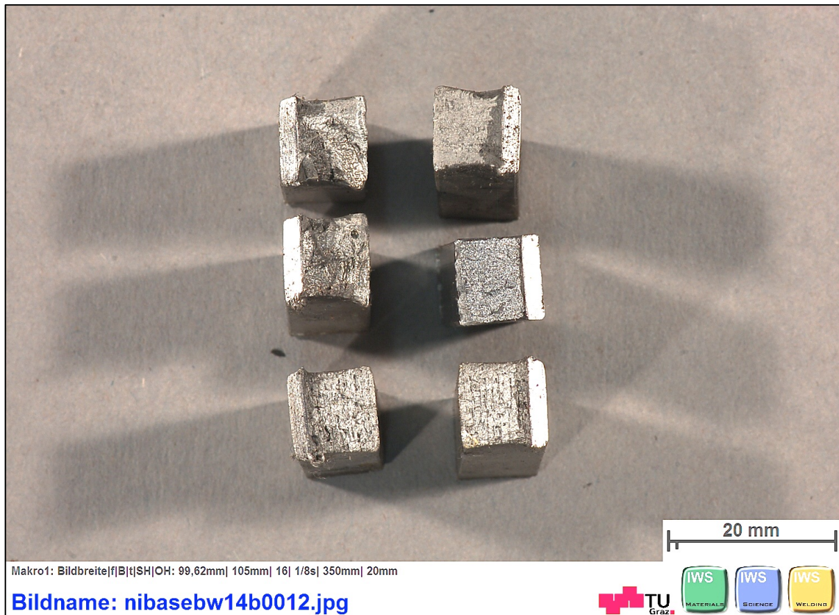
FIGURE 50: CHARPY-V TEST SPECIMEN FRACTURE SURFACES
