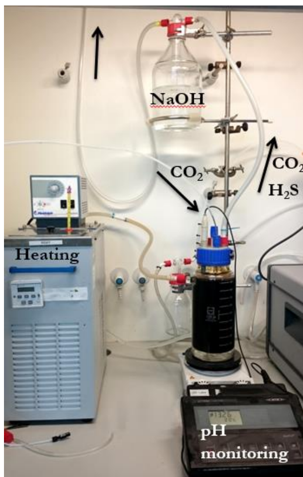
Figure 6-9: Lab scale precipitation experiment with CO 2 as precipitant
