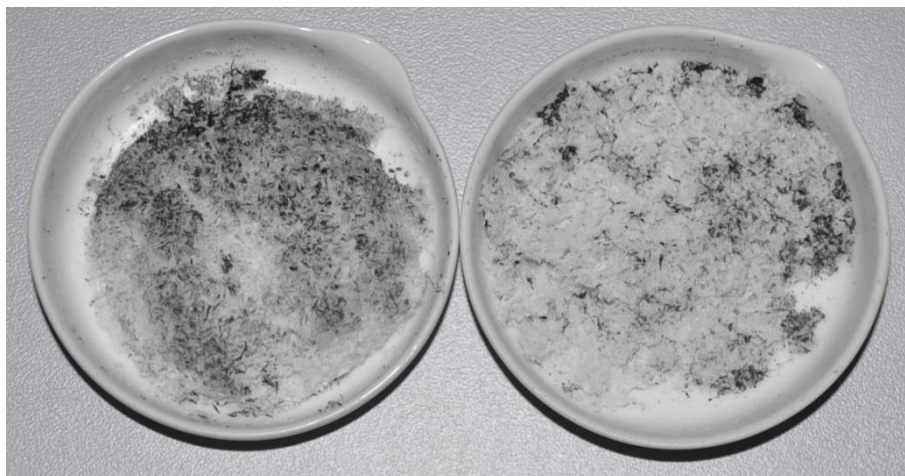
Figure 6-5: Filtrate ash after the incineration
