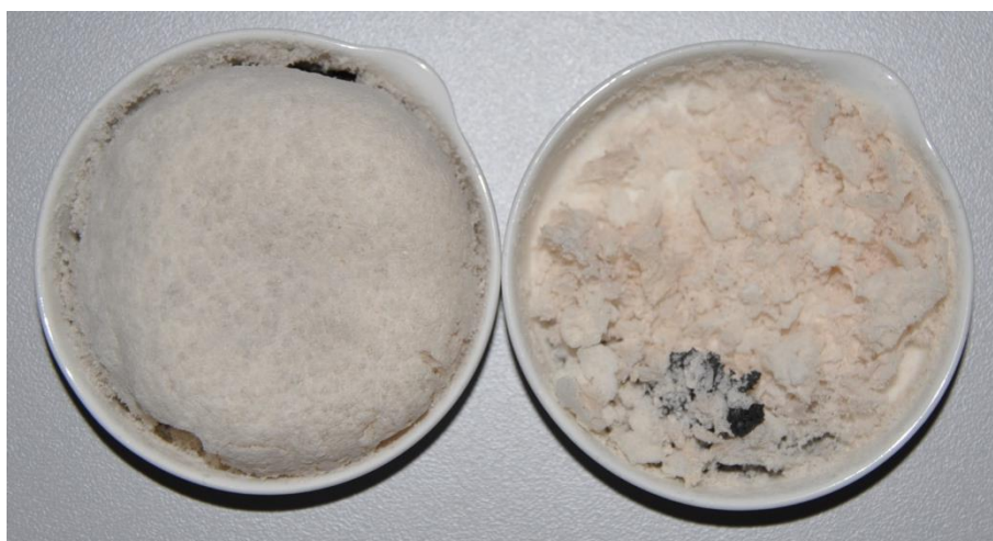
Figure 6-6: Black Liquor ash after the incineration
