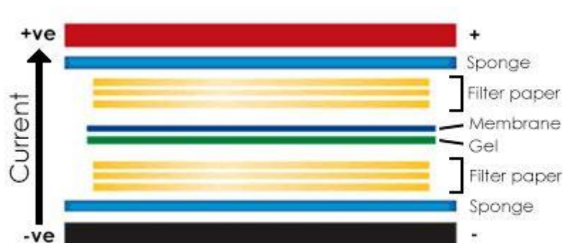
Figure 8: Stack order for protein transfer: Arrangement of the membrane and the gel in the transfer plate, ready for the transfer [34].
