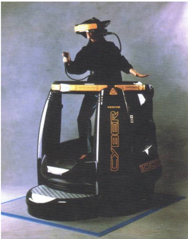
Figure 2.3: Standing user inside the Virtuality system, wearing the Visette
