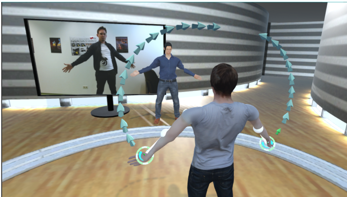
Figure 4.5: The instructions as seen by the user in 3PP with three different instruction methods turned on. Visible are the 3D arrow glyphs, the video instruction and a virtual trainer as an avatar.
