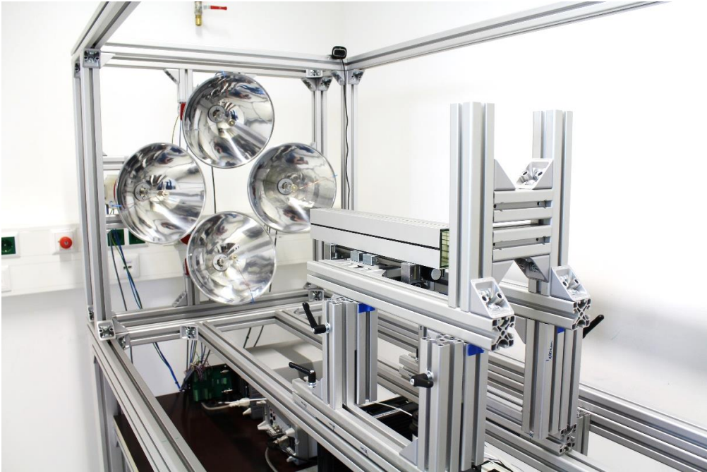
Figure 72: The assembled HFSS with measurement table and light guide tunnel.
