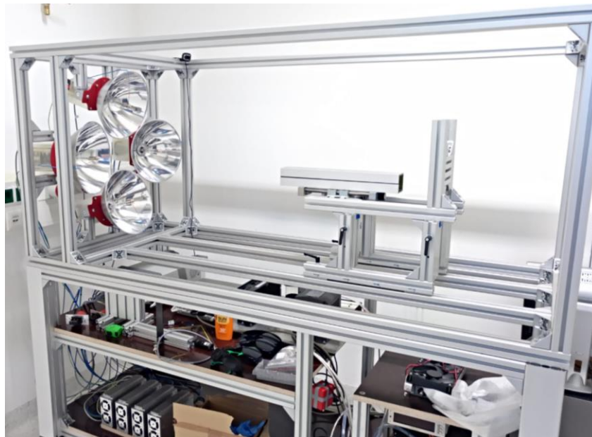
Figure 84: The final assembled HFSS.
