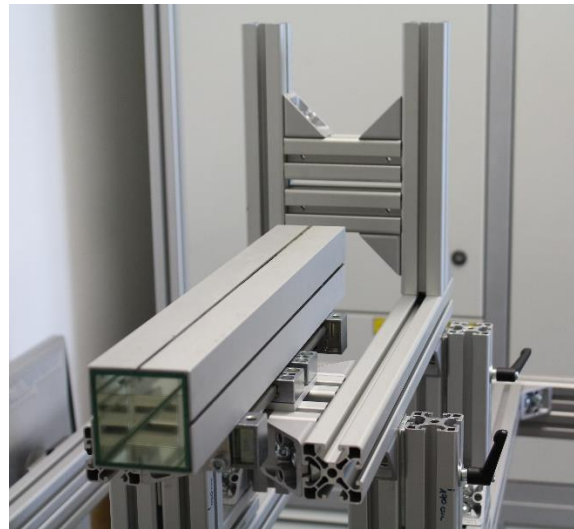
Figure 61: Moveable measurement table with the light guide.
