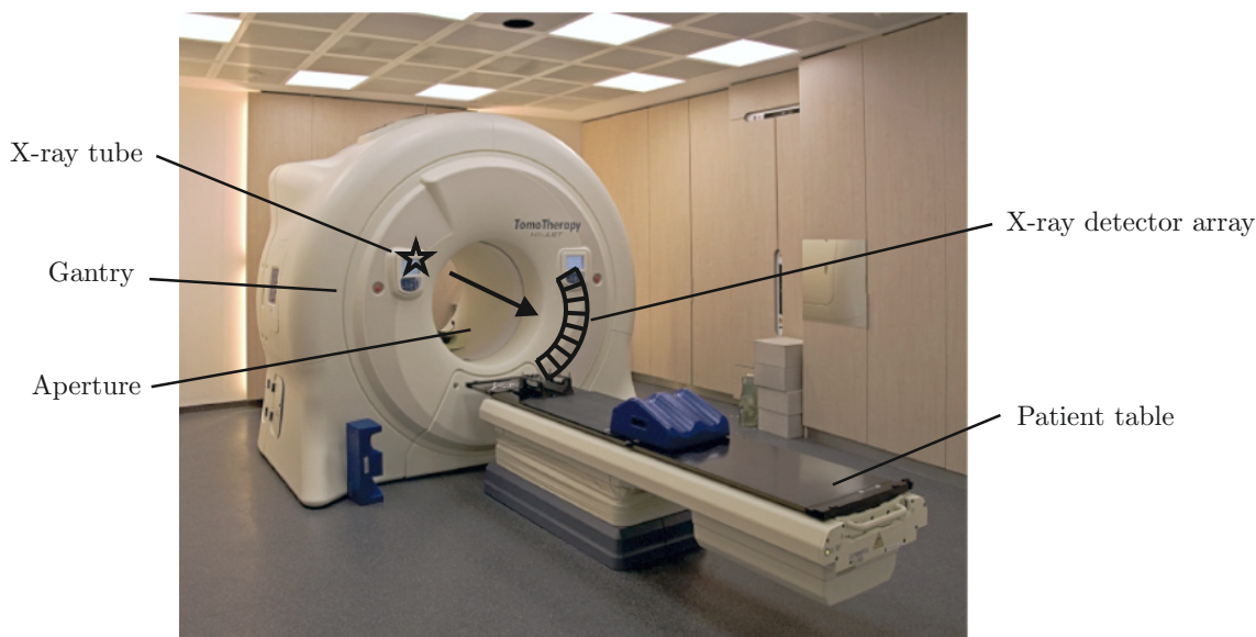
Figure 2.3: A CT scanner with additional visualizations and labels. 4
