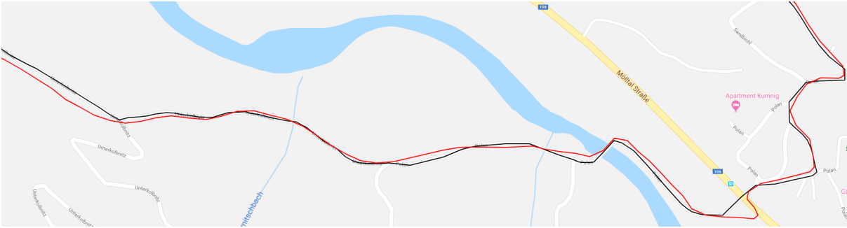
Figure 4.5: The red track is the path using the original GPS coordinates and the black track is the mapped path using the Google Map to Road API and the interpolation option.
