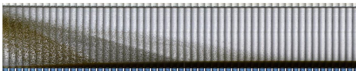
Fig. 8-10: Settling curves of POM particles at \varepsilon_0 = 0.05 in water + 30 wt% PEG-4000; recorded with 0.5 second screen shot technique
