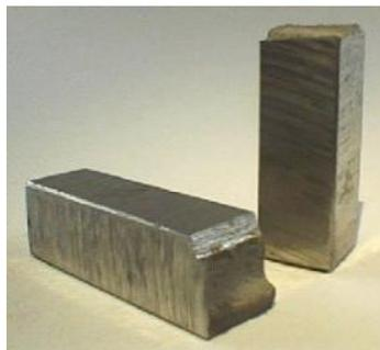
Figure 5.16 – Brittle Fracture of Steel broken at  $-190^{\circ}C$ . *Courtesy of Internet Microscope for Schools.*
