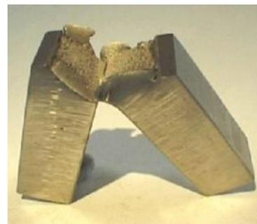
Figure 5.17 – Ductile Fracture of Steel broken at  $-20^{\circ}C$ . *Courtesy of Internet Microscope for Schools.*
