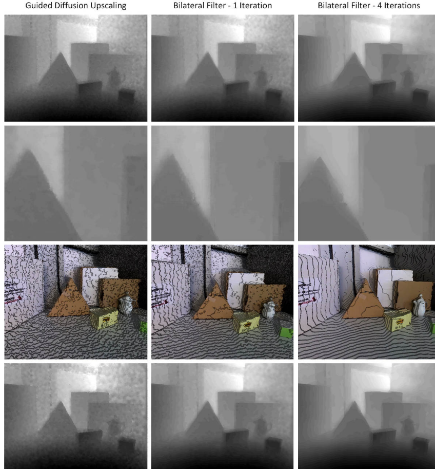
Figure 5.15: The joint bilateral filter [Kop+07] in comparison with the guided diffusion filter. From top to bottom: Depth image; Zoomed depth image; 3D surface mesh; Sensor fusion result with reduced original depth resolution
