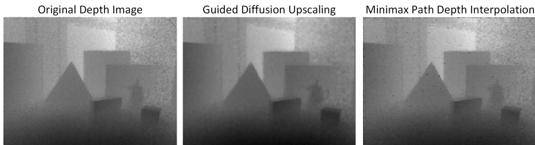
Figure 5.17: The results of the minimax path-based depth interpolation [Dai+15], compared to the original depth image and the proposed guided diffusion upscaling method
