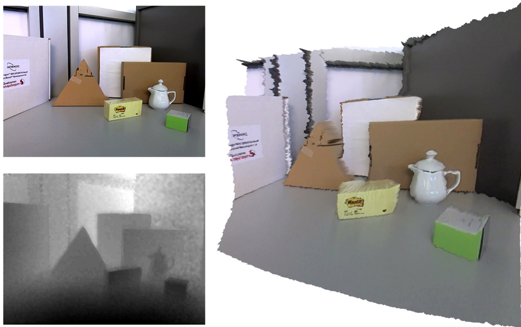
Figure 5.1: Left: Fused color and depth image; Right: 3D surface mesh
