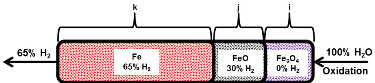
Figure 31: Simplified schema of steam and hydrogen concentration during oxidation after incomplete reduction in reversed flow operation; solid species in the illustration represent the educts of the corresponding reaction.
