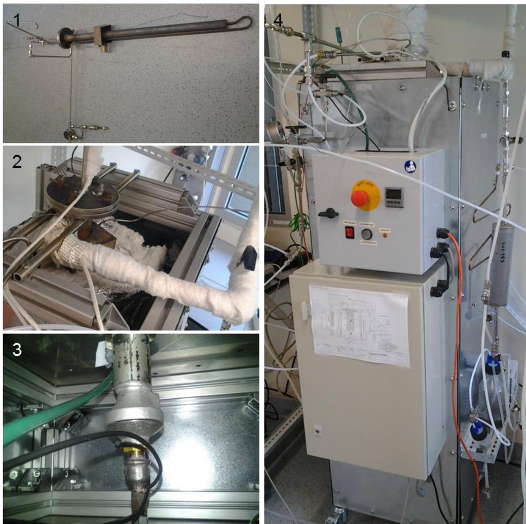
Figure 28: The multi-fixed-bed reactor (1), top section of the prototype (2), gas burner (3) and the complete flex fuel reformer prototype (4).
