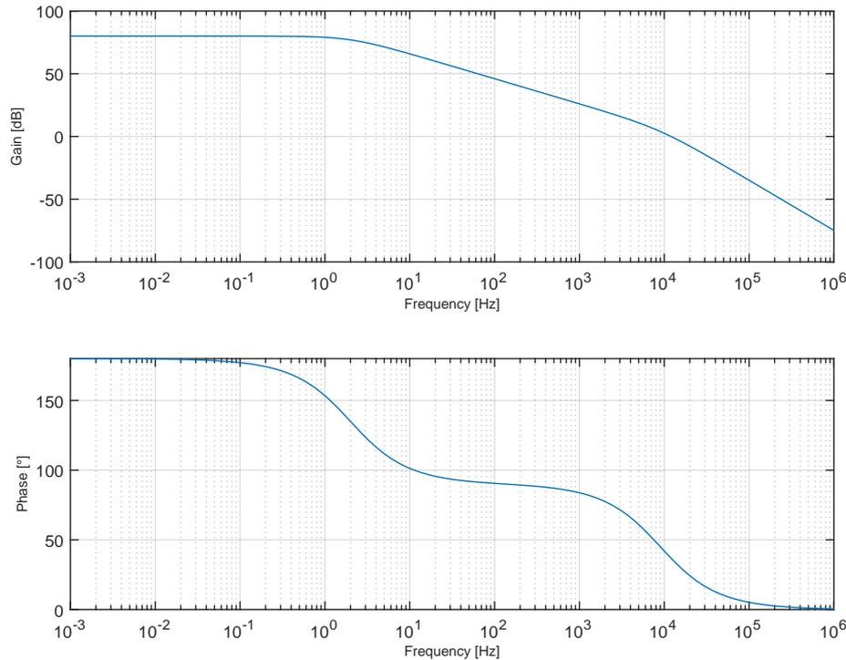
FIGURE 5.5: Calculated Bode diagram for the amplifier including sense transistor. The Bode diagram was based only on the dominant and non-dominant pole.
