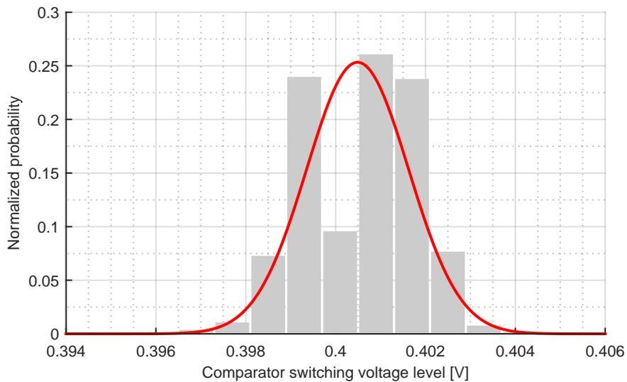
FIGURE 6.13: Distribution of the comparator switching level for the low reference Voltage defined at 400 mV,  $\sigma = 1.1$  mV,  $\mu = 400.5$  mV and  $N = 1000$ .
