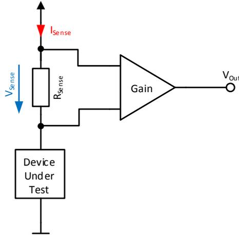
FIGURE 2.3: Architecture of a resistor-based high-side current sensing circuit including amplifier for signal conditioning and/or magnification.
