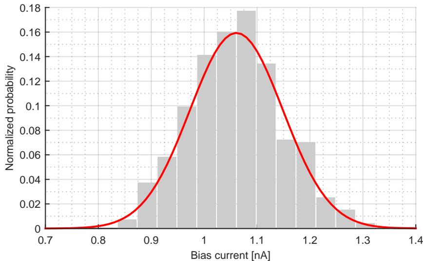
FIGURE 6.1: Distribution of the bias current at 4 V supply voltage,  $\sigma = 87.945$  pA,  $\mu = 1.052$  nA and  $N = 1000$ .
