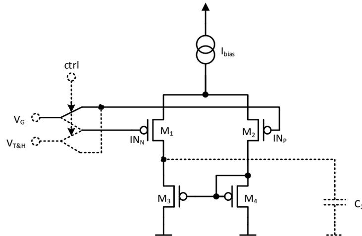
FIGURE 5.17: Output amplifier with load capacitor for integration. The input switches are changing the input signal after each half period of the system clock period.
