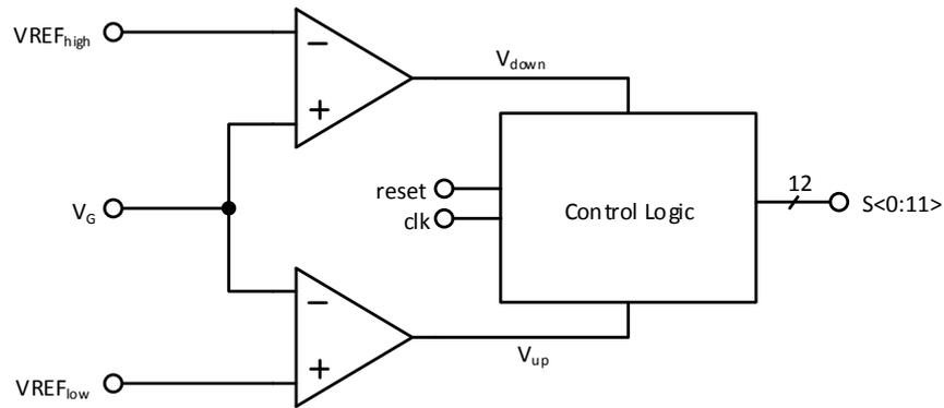
FIGURE 5.6: Overview of the stage selection including comparators and control logic for the generation of the thermometer code based on a 4-bit counter.
