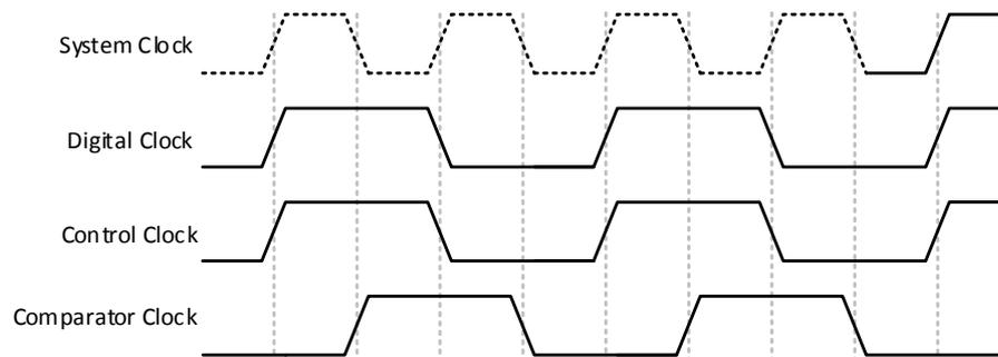
FIGURE 5.7: Timing diagram of the available clock signals including system, digital, control and comparator clock.
