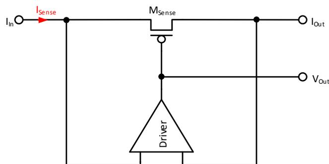
FIGURE 2.6: Gate back current sensor including driver and sense transistor.  $M_{sense}$  is controlled by the driver to work inside the linear region.
