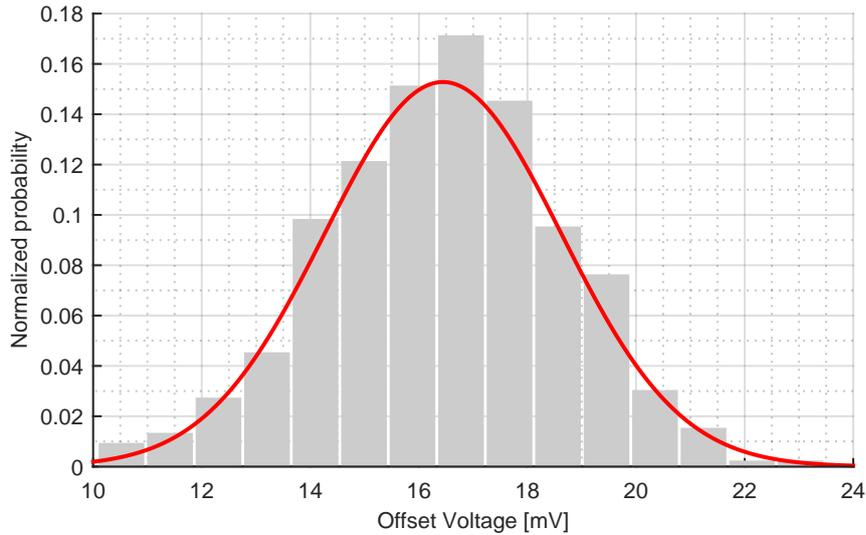
FIGURE 6.6: Distribution of the offset voltage at 2 V supply voltage,  $\sigma = 2.177$  mV,  $\mu = 16.4433$  mV and  $N = 1000$ .
