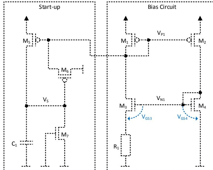
FIGURE 5.1: Basic architecture of the reference current generation including start-up circuit [26].
