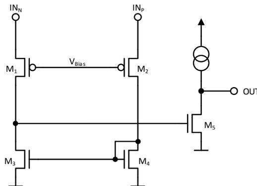
FIGURE 5.4: Input amplifier for the sense element. Basic architecture consists of an input common gate stage with current mirror load followed by a common source stage.
