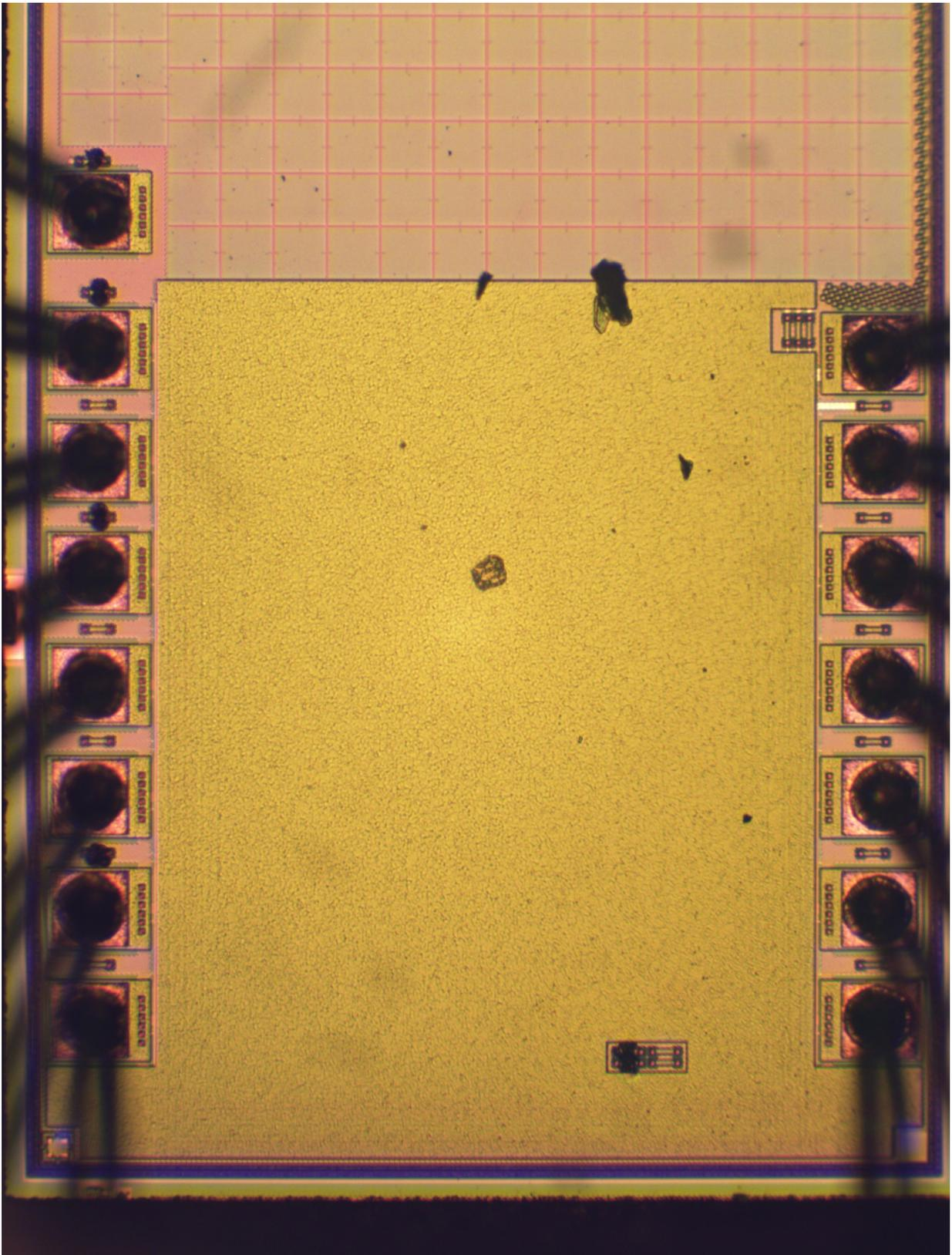
FIGURE 7.7: Image of the chip after fabrication. A part of the photo diode arrays, bonding pads as well as the fuses are visible. In the lower right corner, two fuses can be seen after cutting. The remaining circuits are not visible due to additional layers on top of the metal stack.
