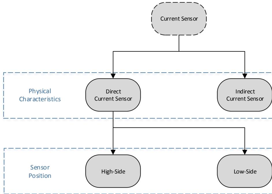
FIGURE 2.1: Overview of current sensor classifications based on their physical measurement principle as well as their actual position inside the system [8].
