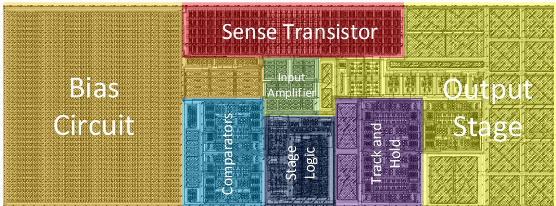
FIGURE 7.2: Layout for the current sensor including all major circuit blocks. The resulting area is mainly caused by the bias circuit resistor, sense transistor as well as output stage capacitors.
