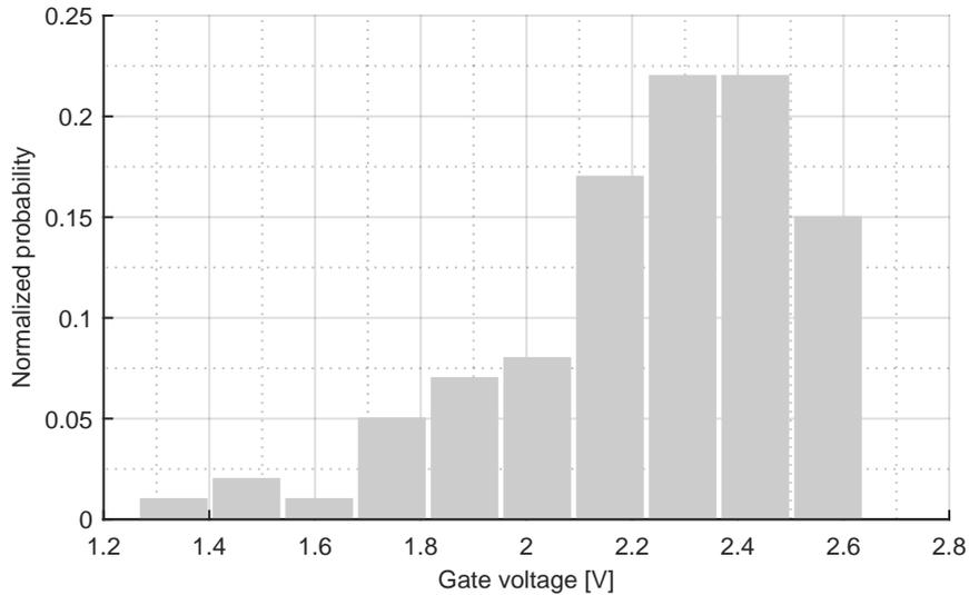
FIGURE 6.21: Gate voltage distribution for a supply level of 4 V with  $\sigma = 0.2738$  V,  $\mu = 2.2392$  V and  $N = 100$ .
