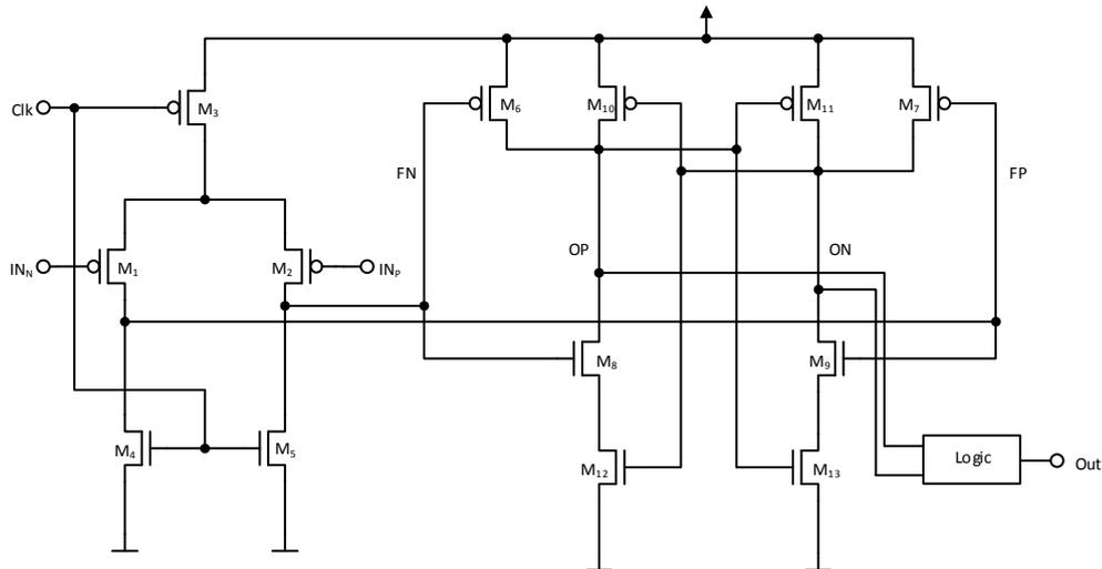
FIGURE 5.10: Comparator with a PMOS input preamplifier stage followed by a latch. The logic for the output signal generation is based on a RS-Flip-Flop.
