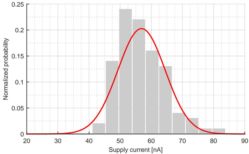
FIGURE 6.25: Current consumption at 4 V analog supply with  $\sigma = 7.585$  nA,  $\mu = 56.86$  nA and  $N = 100$ .
