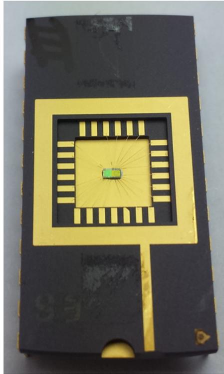
FIGURE 7.6: Image of the packaged test chip, where the die itself, the bonding wires as well as the photo diodes can be seen.
