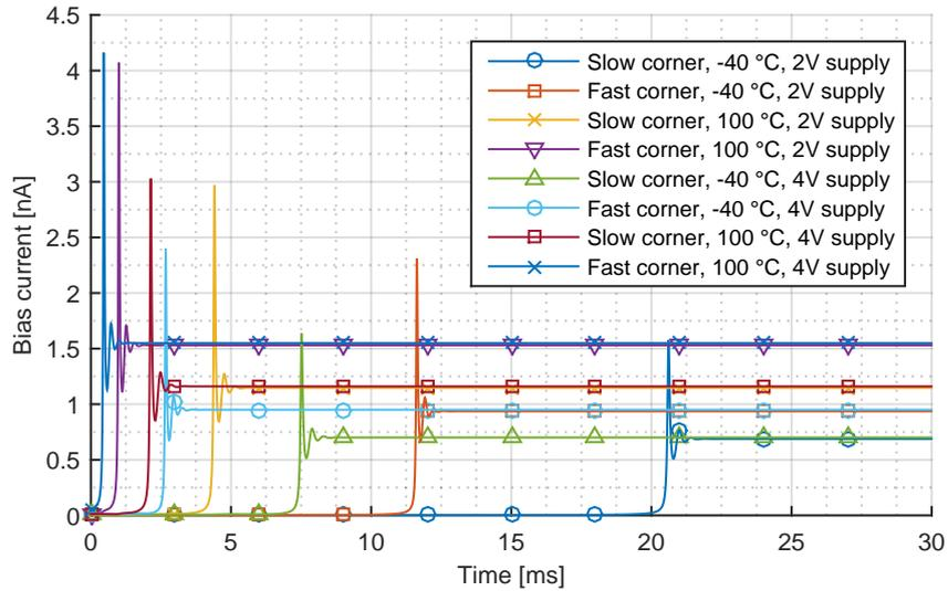
FIGURE 6.3: Start-up behavior of the bias circuit depending on the process corner, supply voltage and temperature. The system start-up time is, under worst condition (slow corner and lowest temperature which results in the smallest leakage current), approximately below 20 ms.
