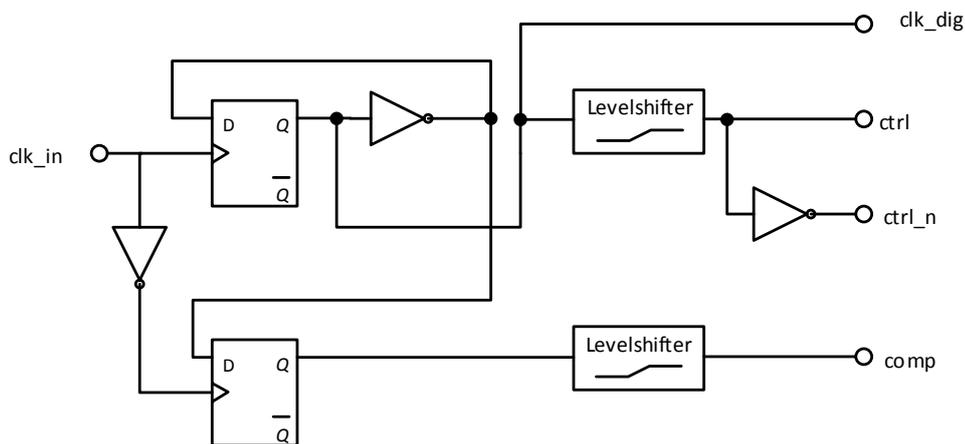
FIGURE 5.8: Clock generation circuit based on the given system clock. The output inverter for the ctrl\_n signal must be an analog inverter due to the higher supply voltage after the level shifter.
