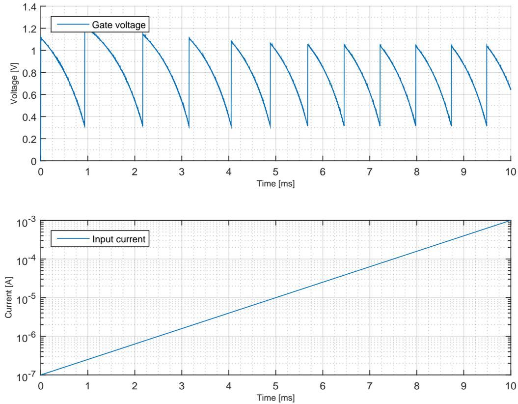
FIGURE 6.16: Gate and comparator reference voltages for an input current range from 100 nA to 1 mA with a logarithmic source.
