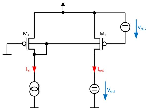
FIGURE 3.1: PMOS bulk-driven current mirror with  $M_1$  inside the linear region and  $M_2$  inside saturation.
