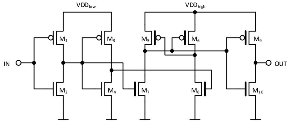
FIGURE 5.15: Level shifter for the interface between the low and the high supply voltage domain. Transistors marked with a thicker gate are analog devices for the high supply domain.
