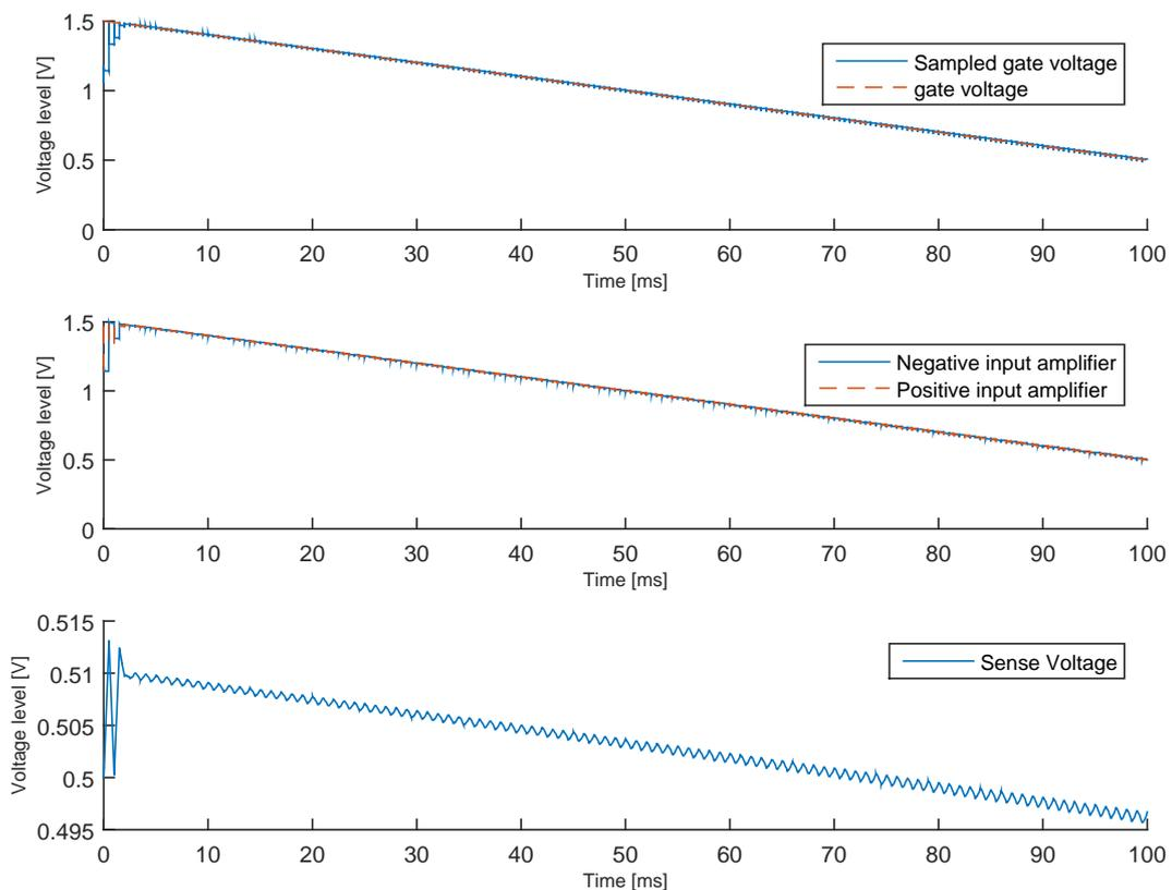
FIGURE 6.19: Output voltage of the control signal generation including the gate and sampled voltage, negative and positive amplifier input as well as output signal. The drift of the sense voltage due to mismatches inside the integrator can be seen.
