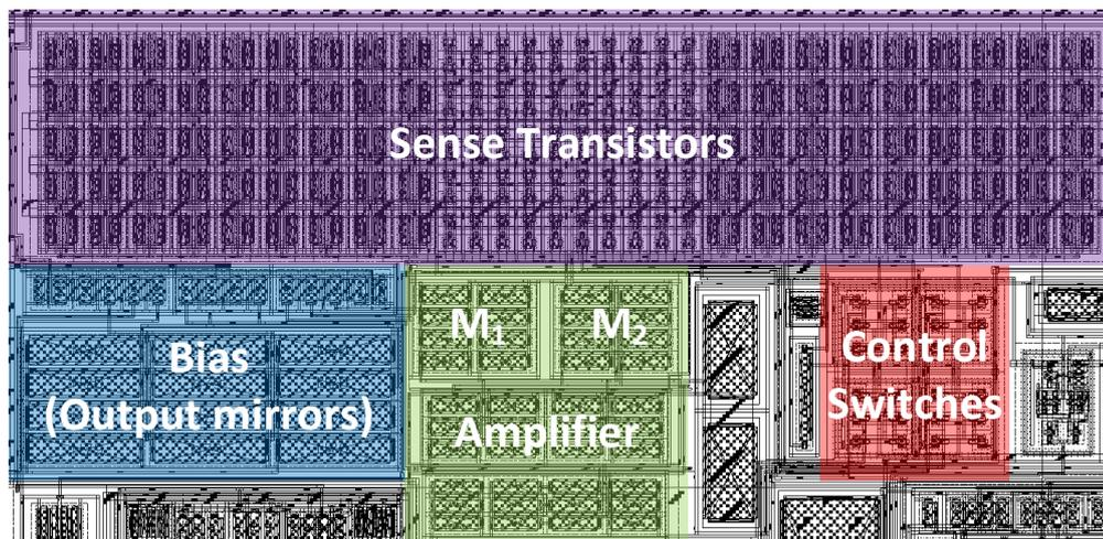
FIGURE 7.3: Layout for the sense transistor including control switches as well as the input amplifier and the output mirror transistors from the bias circuit.
