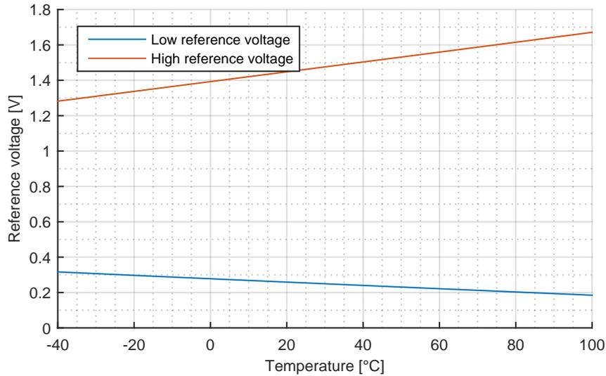
FIGURE 6.11: Temperature dependency of the high and low reference voltages.
