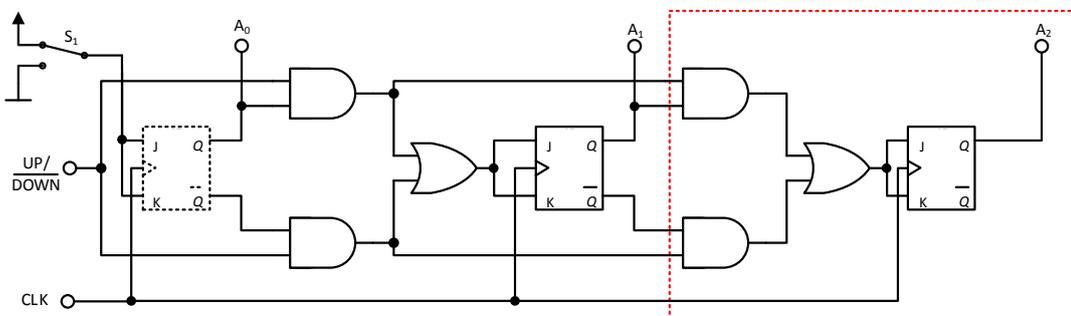
FIGURE 5.13: Block diagram for the bidirectional counter where only three bits are shown for simplicity. The required stage for one bit is marked red. This stage needs to be copied for each additional bit.
