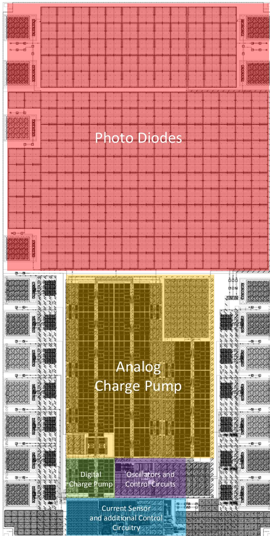
FIGURE 7.1: Top level layout of the test chip including photo diodes, charge pump as well as the proposed current sensor.
