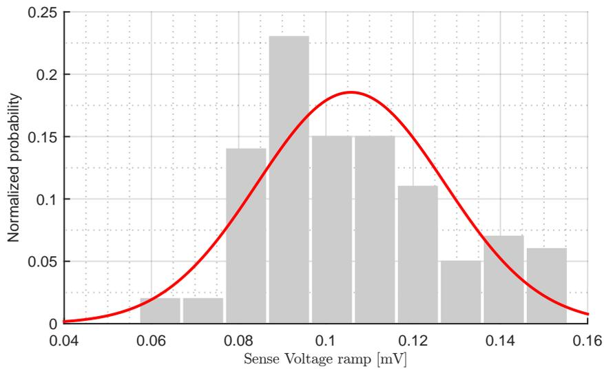
FIGURE 6.24: Sense voltage step during a peak detection for a supply level of 2 V with  $\sigma = 21.5\text{mV}$ ,  $\mu = 105.8\text{mV}$  and  $N = 100$ .
