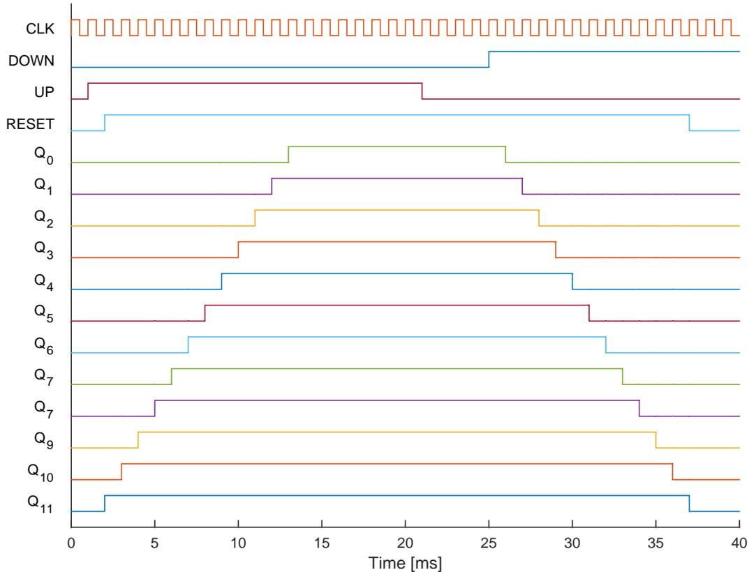
FIGURE 6.14: Timing diagram for the bidirectional counter during the up and down phase. Signals are normalized to logic true and false values.
