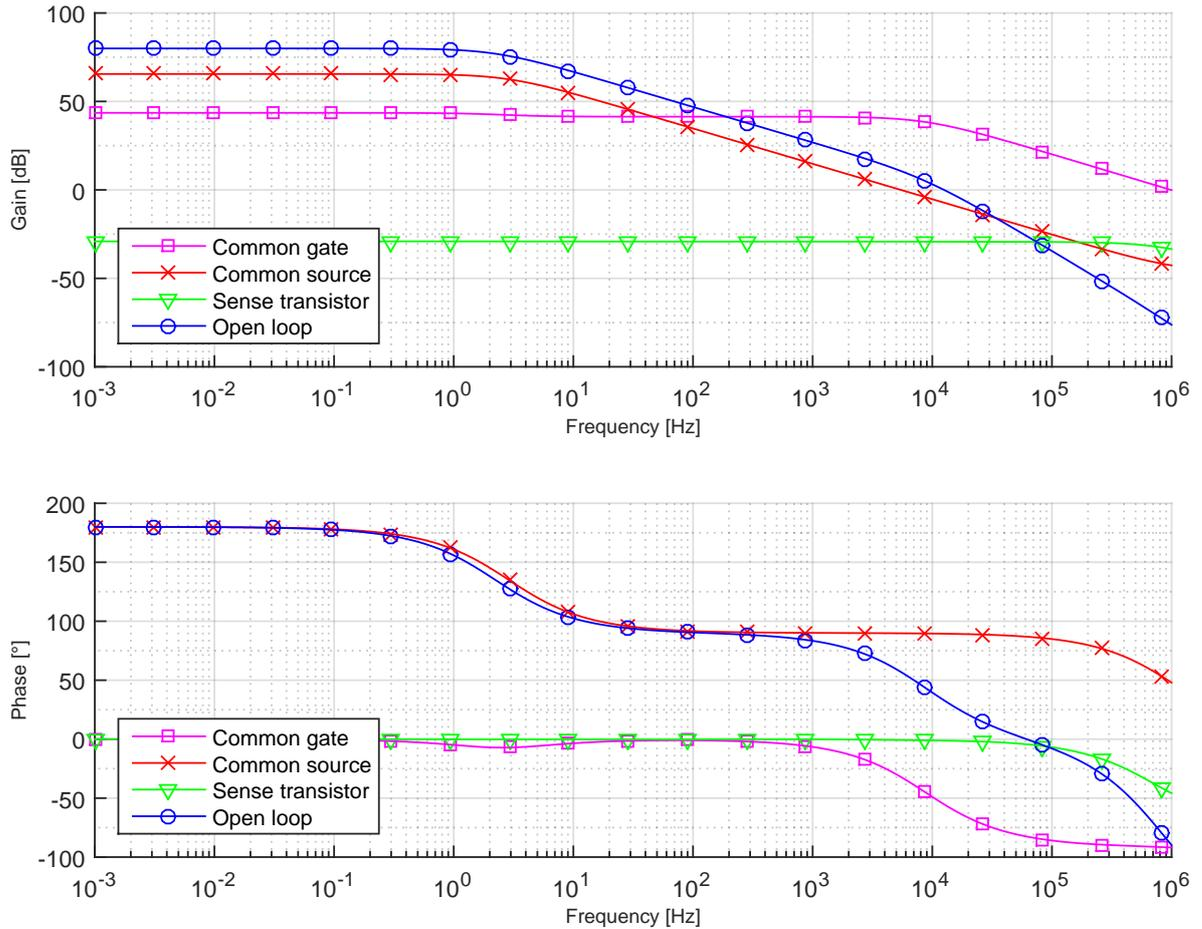
FIGURE 6.7: Bode diagram of the separate amplifier stages. Common gate, common source, sense transistor as well as open loop are shown separately.
