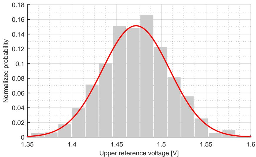
FIGURE 6.10: Distribution of high reference voltage at 2 V supply,  $\sigma = 37.65 \text{ mV}$ ,  $\mu = 1.4716 \text{ V}$  and  $N = 1000$ .
