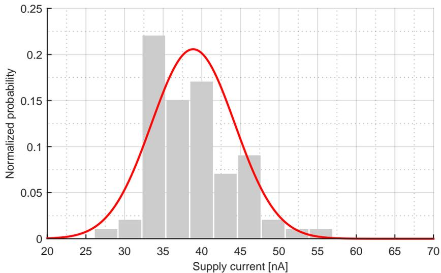
FIGURE 6.26: Current consumption at 2 V analog supply with  $\sigma = 5.398$  nA,  $\mu = 38.9$  nA and  $N = 100$ .
