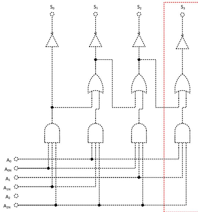
FIGURE 5.14: Section of the combinational logic for the first 4 bits of the thermometer code. The required cells for one additional bit are marked red.
