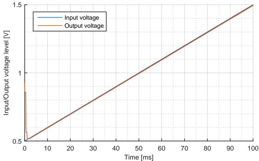
FIGURE 6.17: Input and output voltage of the track and hold stage including start-up behavior as well as the possibly occurring input voltage range.
