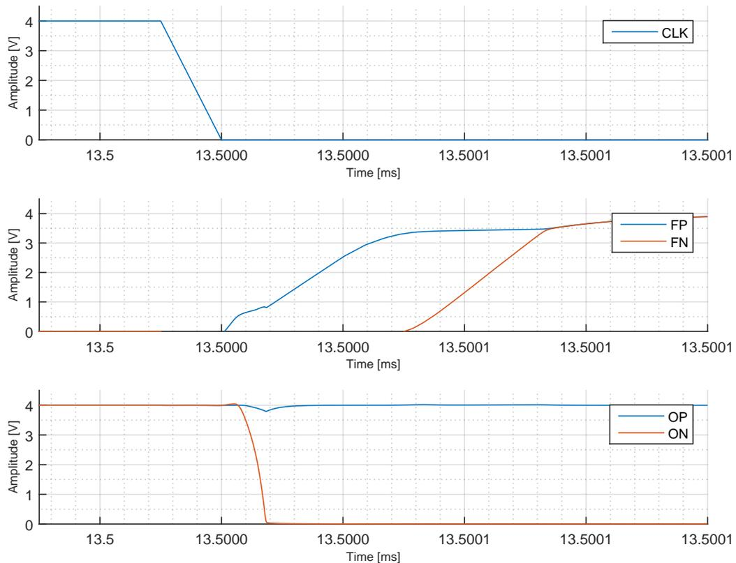
FIGURE 5.11: Internal comparator signals during one comparison phase at the falling clock edge. Internal nodes FN, FP at the output of the preamplifier as well as OP and ON at the output of the comparator are shown.
