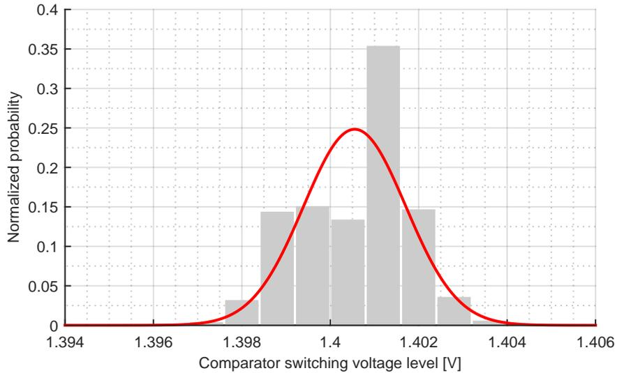
FIGURE 6.12: Distribution of the comparator switching level for the high reference voltage defined at 1.4 V,  $\sigma = 1.2$  mV,  $\mu = 1.4006$  V and  $N = 1000$ .
