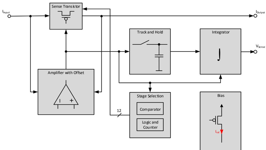
FIGURE 4.1: Block diagram of the complete current sensor based on the gate back architecture with additional control signal generation and bias circuitry. Orange marked blocks are related to the current sensor itself whereas blue marked blocks are related to the control signal generation.
