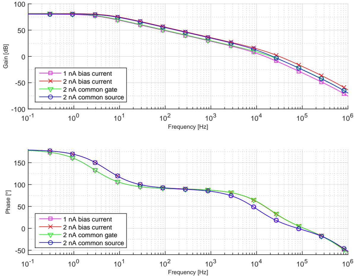
FIGURE 6.8: Bode diagram for the open loop circuit under different bias current scenarios. In case it is not explicitly mentioned, all stages are bias with 1 nA. The effect of the different bias currents can be mainly seen in a shift of the pole, whereas the open loop gain is in a first order independent from the bias current.
