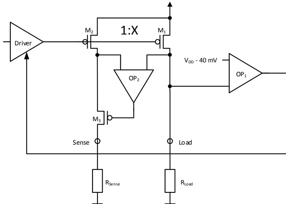
FIGURE 3.2: Typical application for a gate back circuit using a regulated gate driver for drain source voltage regulation. The load transistor  $M_1$  and the sense transistor  $M_2$  are driven by  $OP_1$  in a gate-back configuration.
