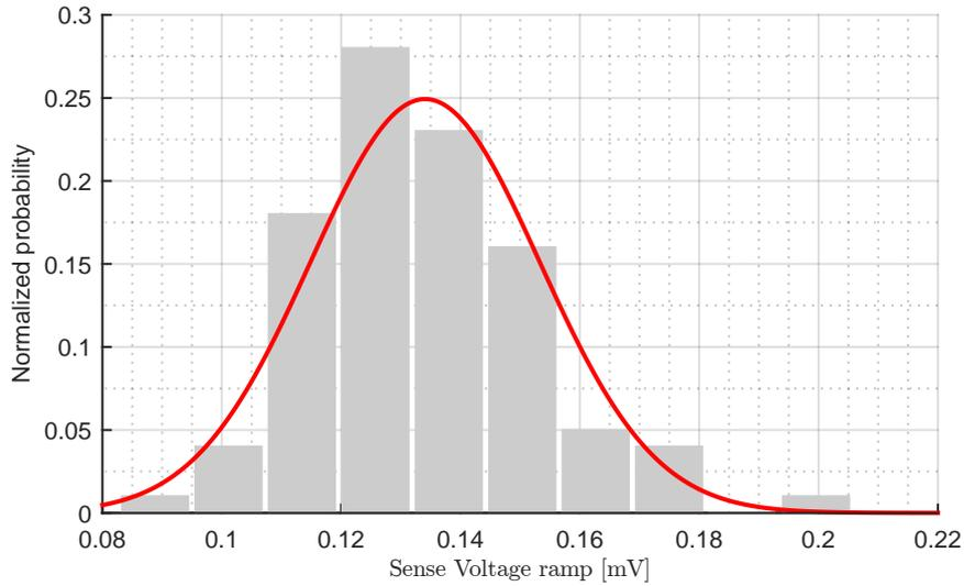
FIGURE 6.23: Sense voltage step during a peak detection for a supply level of 4 V with  $\sigma = 19.2\text{mV}$ ,  $\mu = 134.1\text{mV}$  and  $N = 100$ .
