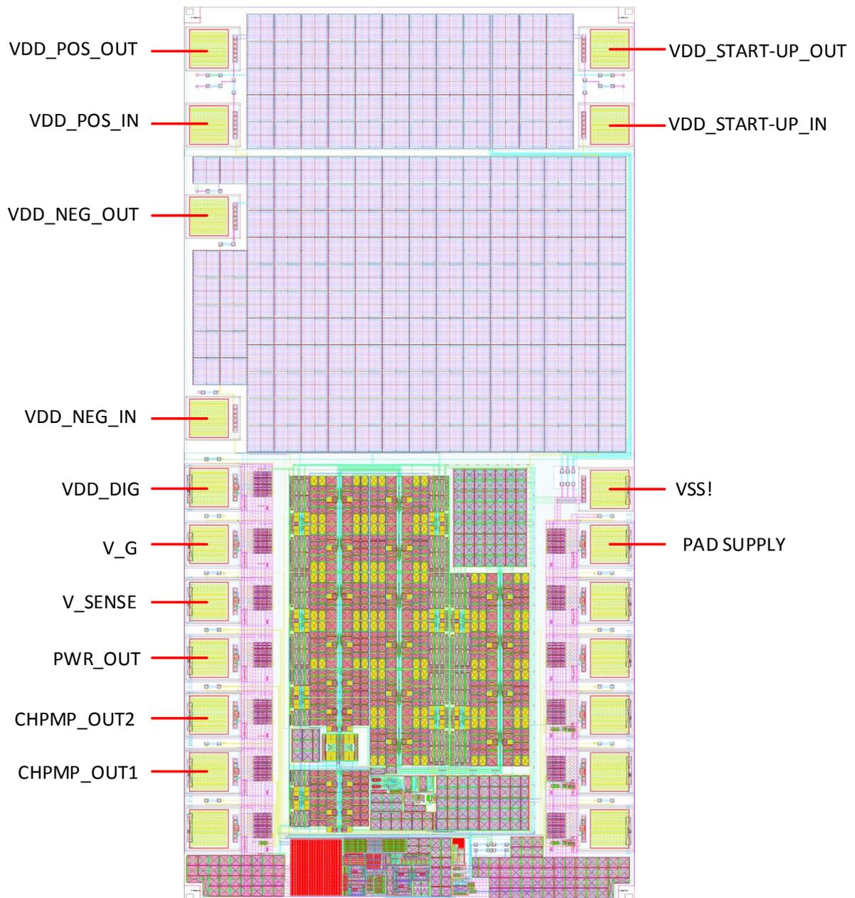
FIGURE 7.8: Position and signal name for the most important bonding pads. V\_G is the gate voltage of the sense transistor and V\_SENSE the output voltage of the control signal generation. VDD.DIG and PWR.OUT are the digital and analog supply voltages.
