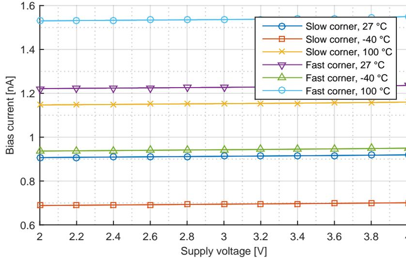
FIGURE 6.2: Temperature and supply voltage dependency of the bias current over process corners. It can be seen that the supply voltage variation can be neglected compared to the process corner and temperature variations.
