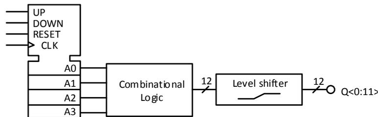
FIGURE 5.12: Block diagram for the control logic. Based on a four-bit counter, the required 12 control bits were generated by a combinational logic and then shifted to the higher supply domain.
