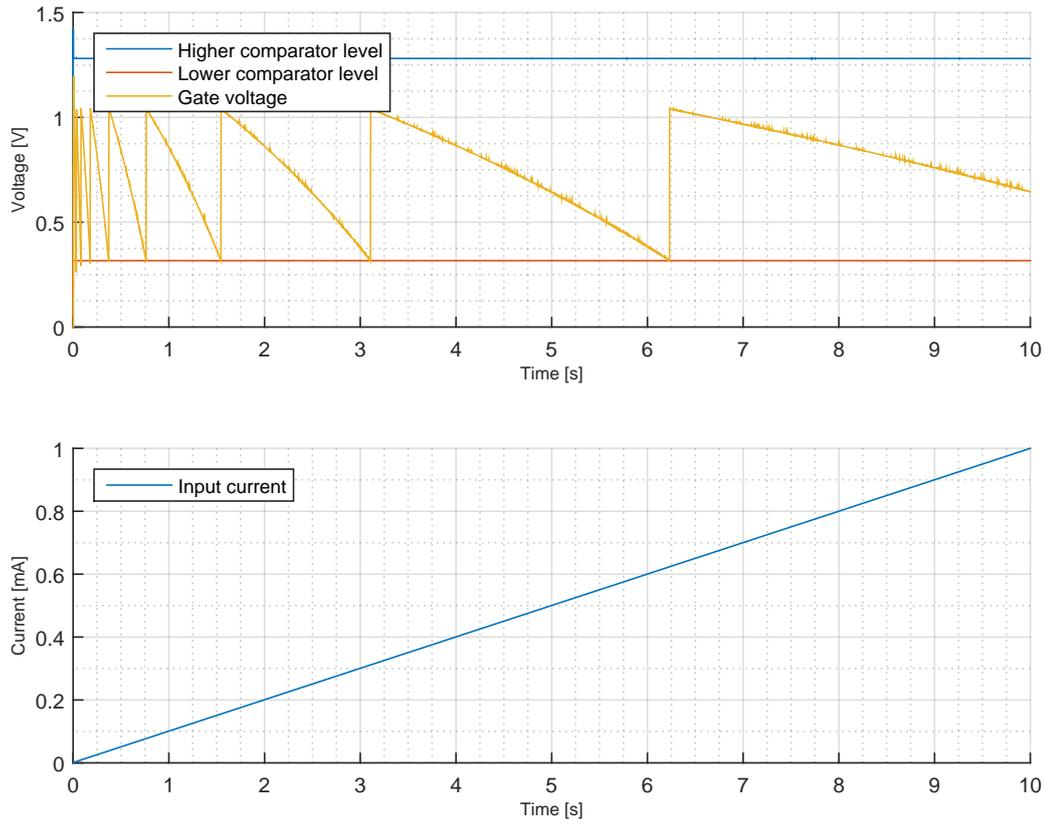
FIGURE 6.15: Gate and comparator reference voltages for an input current range from 100 nA to 1 mA.
