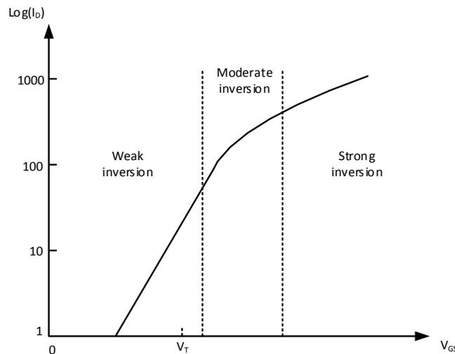
FIGURE 2.7: Inversion regions for a MOS transistor including strong, moderate and weak inversion. The drain current dependency on the gate source voltage is shown with a logarithmic y-axis.
