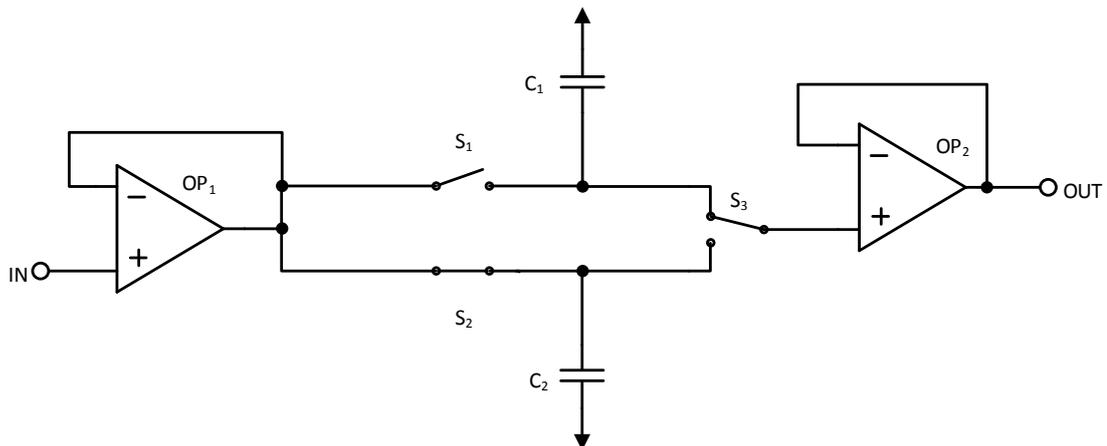
FIGURE 5.16: Track and hold circuit including input and output buffers. The capacitors  $C_1$  and  $C_2$  are each for one half of the system clock period.  $S_3$  switches between the currently held signal.
