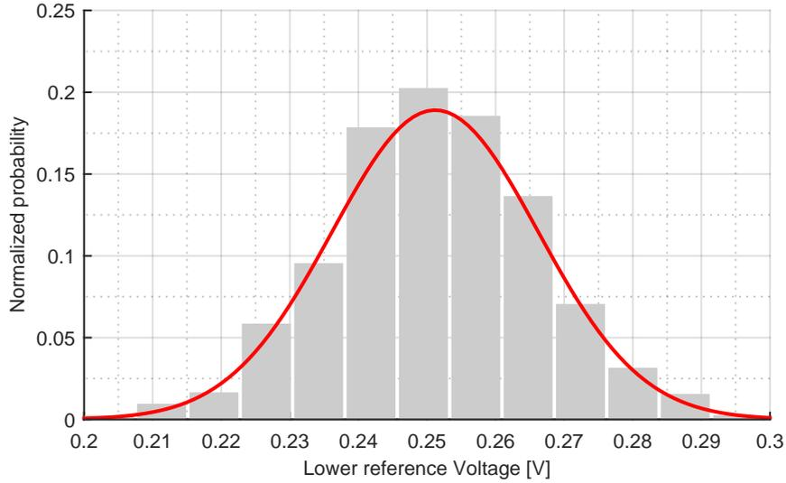
FIGURE 6.9: Distribution of the low reference voltage at 2 V supply,  $\sigma = 15.03 \text{ mV}$ ,  $\mu = 251.2 \text{ mV}$  and  $N = 1000$ .
