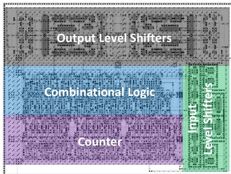
FIGURE 7.4: Layout of the control logic including counter, combinational logic and level shifters.
