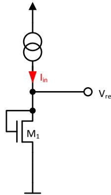
FIGURE 5.9: Reference voltage generation using a current source with a diode-connected transistor as load.
