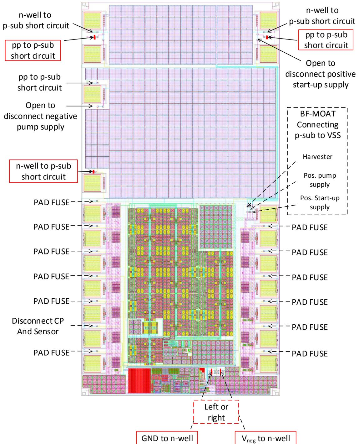
FIGURE 7.9: Detailed position and short explanation of the fuses including the fuse to disconnect the charge pump from the current sensor. Red marked fuses must be destroyed after fabrication to guarantee circuit functionality. PAD FUSES are fuses to disconnect the bonding pads from the circuitry.
