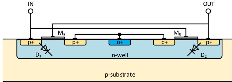
FIGURE 5.3: Cross section of the PMOS sense transistor including parasitic diodes at the input and output of the sense element.
