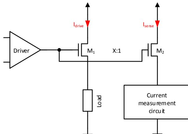
FIGURE 2.4: Current sensor example for high-side driver including drive ( $M_1$ ) and measurement ( $M_2$ ) transistor with an aspect ratio  $X:1$ .
