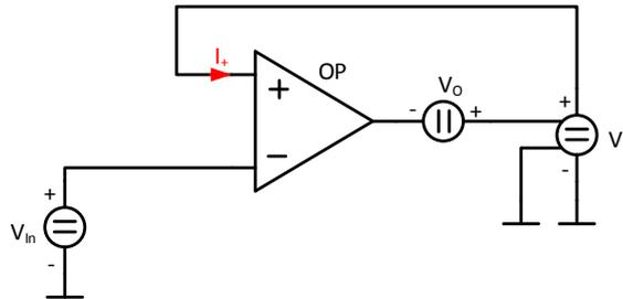
FIGURE 6.5: Basic simulation circuit for the input amplifier without sense element. Additional voltage source  $V_O$  and voltage-controlled voltage source  $V_B$  required for operation.
