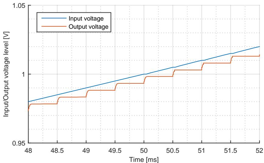
FIGURE 6.18: Detailed view on the input and output signal of the track and hold stage.
