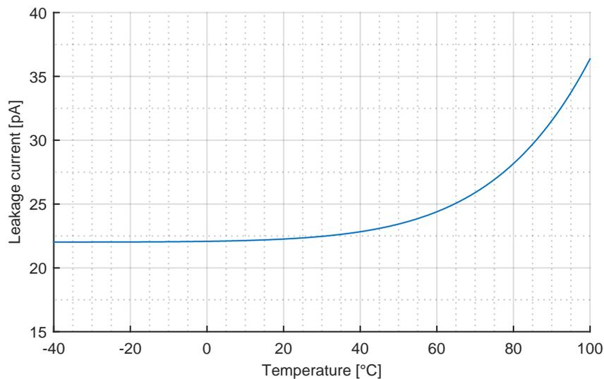
FIGURE 6.4: Leakage current of an NMOS transistor with  $L=2\mu\text{m}$  and  $W=600\text{nm}$  depending on the temperature.
