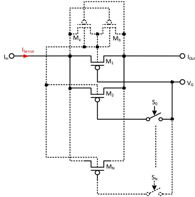
FIGURE 5.2: PMOS sense transistors including bulk regulation and switches for stage selection. In case a certain switch is open, the corresponding gate is connected to the positive supply voltage.
