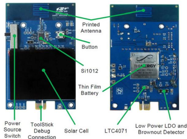
FIGURE 1.1: PCB reference design for a complete wireless sensor node including solar cell, antenna, battery charger system (LTC4071), thin film battery and ultra-low power micro controller unit with integrated transceiver (Si1012) [2].
