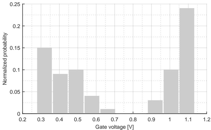
FIGURE 6.22: Gate voltage distribution for a supply level of 2 V with  $\sigma = 0.3342$  V,  $\mu = 0.7304$  V and  $N = 100$ .
