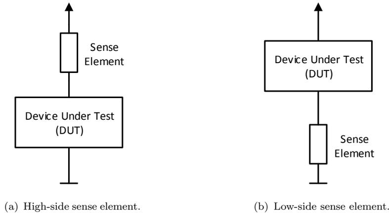
FIGURE 2.2: Basic concept of a high-side and a low-side current measurement. Schematic diagram for the position of the sense element related to the device under test for a high-side (2.2(a)) as well as low-side (2.2(b)) configuration.
