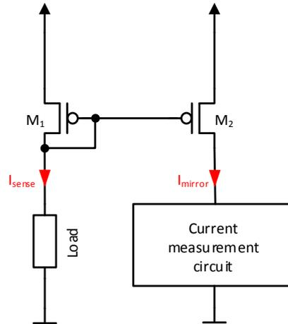
FIGURE 2.5: High-side current sensor using  $M_1$  and  $M_2$  as basic current mirror.
