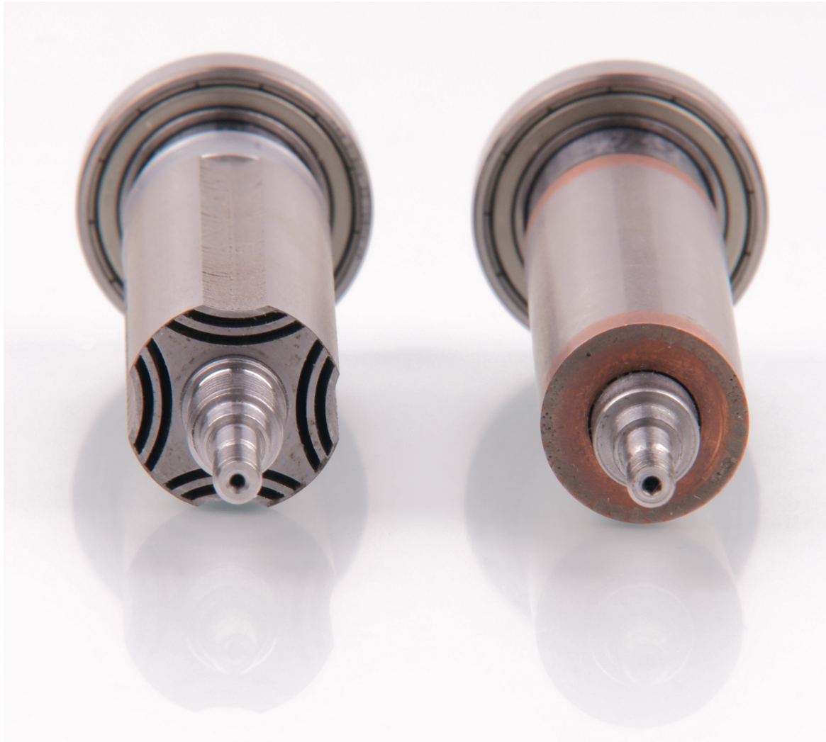
(a) Comparison of the two manufactured rotors (SynRM left and IM right).
