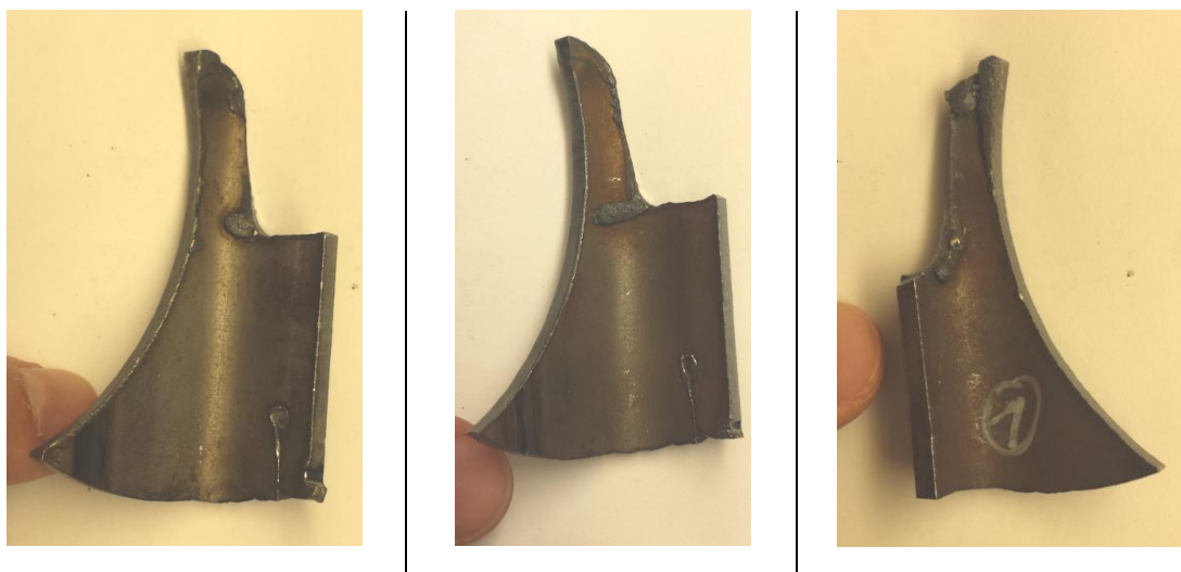
Figure 77: Dross issues when cutting the final part, Source: own illustration
