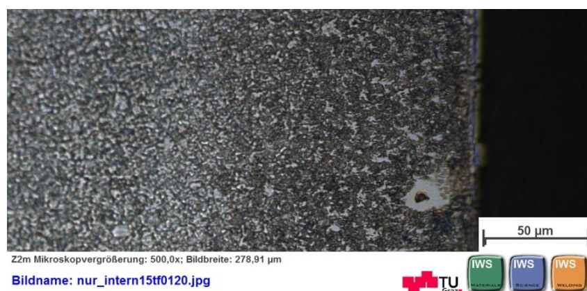
Figure 95: Heat affected zone, 22MnB5 – Laser 2 kW – 200 mms-1, Source: own illustration
