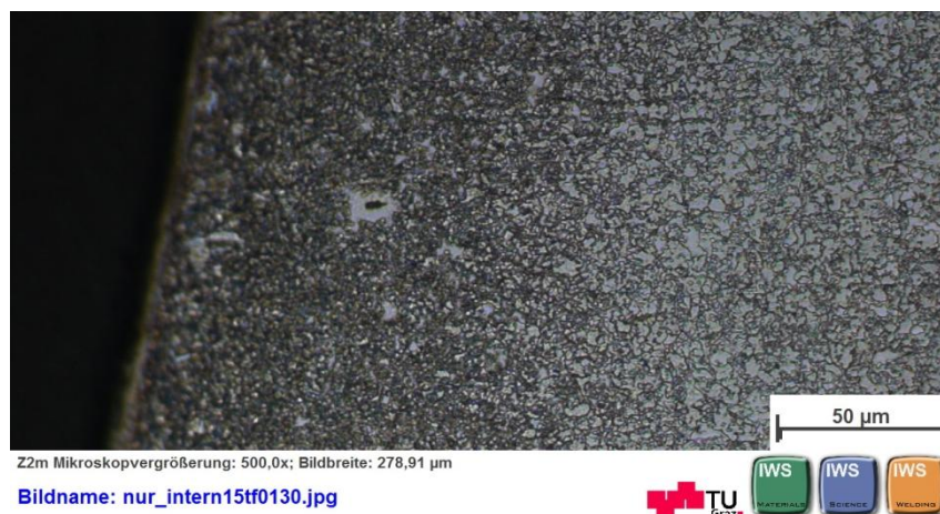
Figure 94: Heat affected zone, 22MnB5 – PMX 55 A – 100 mms-1, Source: own illustration
