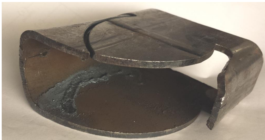
Figure 81: Dross in a tube, Source: own illustration
